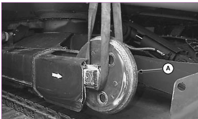
T118321-UN: Remove Front Idler
