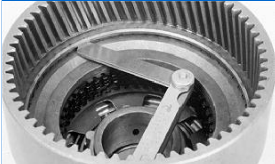
T5985AP-UN: Use A Feeler Gauge To Measure The Distance
