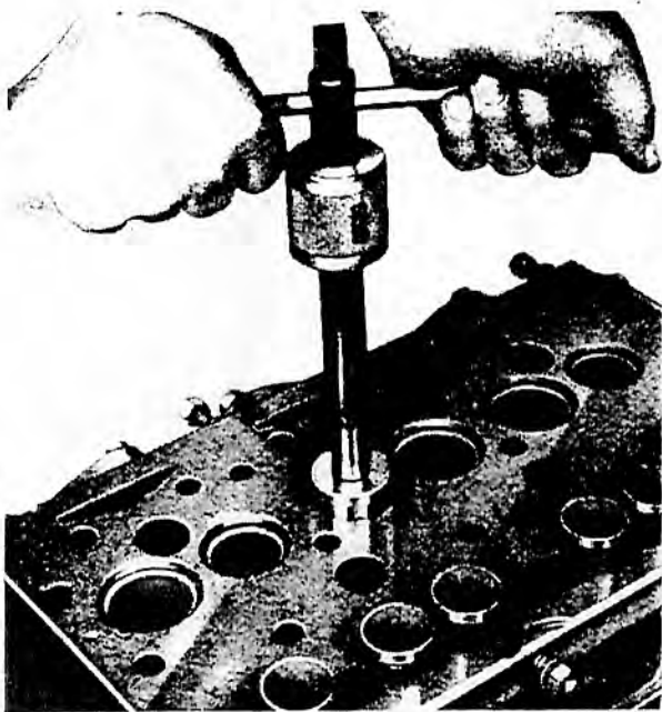
FIGURE 6 RE-CUTTING VALVE SEATS
