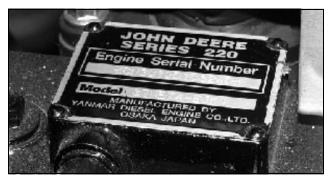
Located on top of the engine rocker cover.
