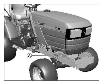
Located on right-hand side of frame beneath the front of the engine.
