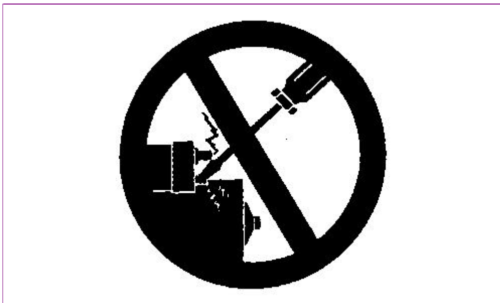
RG5419-UN: Prevent Bypass Starting
