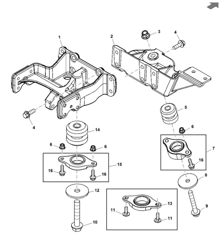
John Deere > Turf And Utility > UTILITY VEHICLE > XUV - UTILITY VEHICLE > XUV Gator Utility Vehicle 855D (Diesel) > 20 ENGINE 3TNV70-ETN173137 > ST562923 - ISOLATOR
