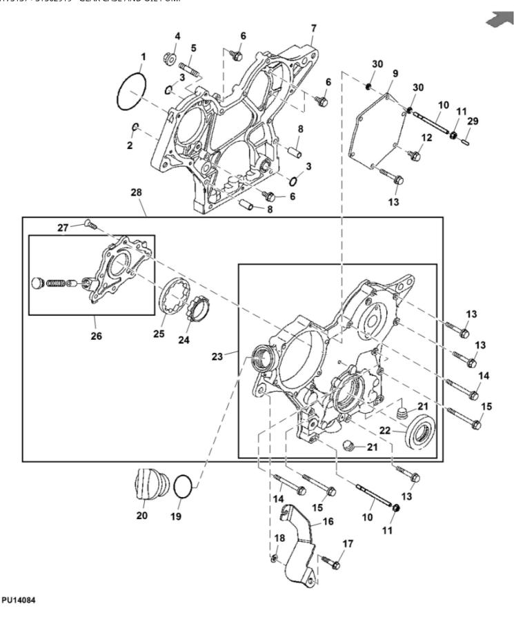
John Deere > Turf And Utility > UTILITY VEHICLE > XUV - UTILITY VEHICLE > XUV Gator Utility Vehicle 855D (Diesel) > 20 ENGINE 3TNV70-ETN173137 > ST562919 - GEAR CASE AND OIL PUMP
