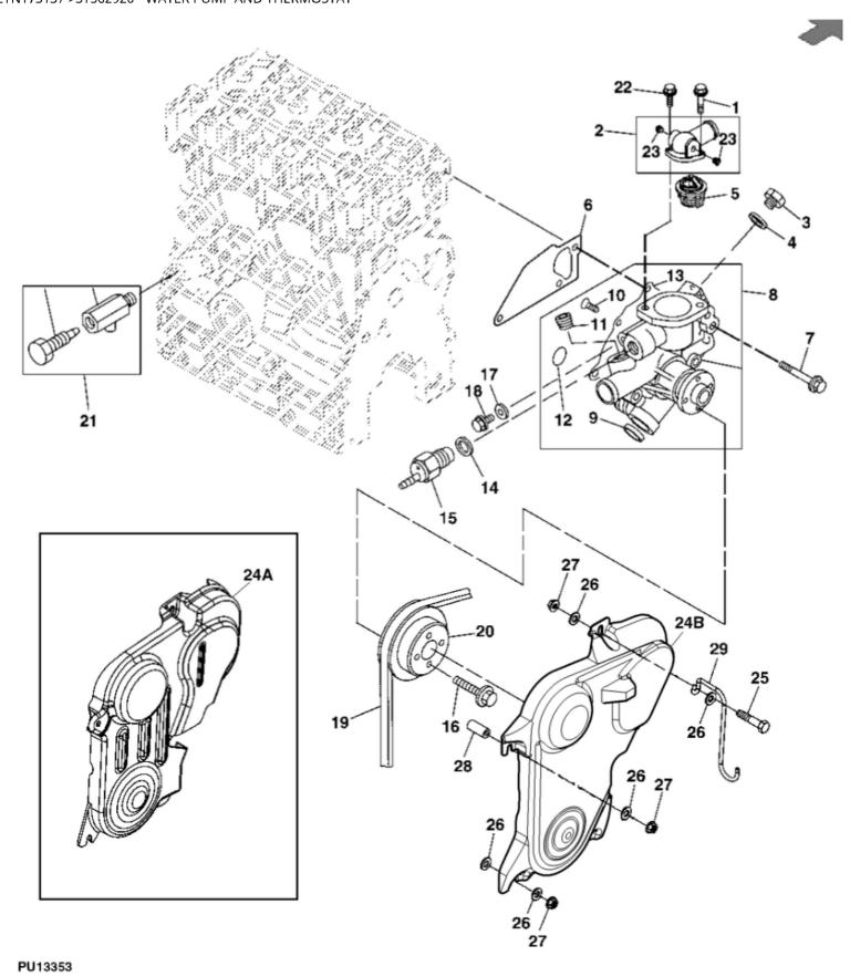
John Deere > Turf And Utility > UTILITY VEHICLE > XUV - UTILITY VEHICLE > XUV Gator Utility Vehicle 855D (Diesel) > 20 ENGINE 3TNV70-ETN173137 > ST562920 - WATER PUMP AND THERMOSTAT
