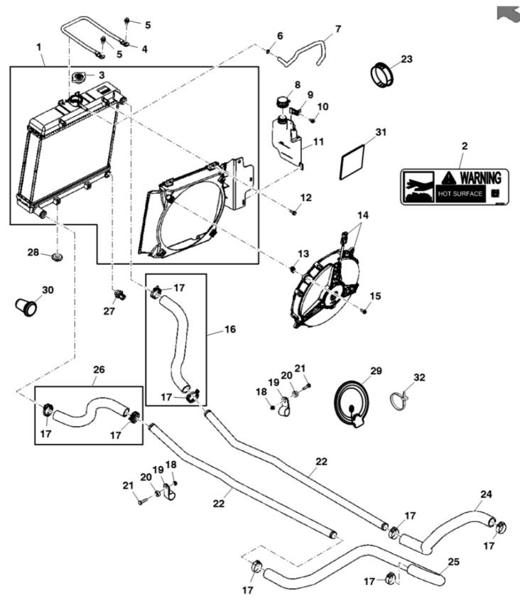
John Deere > Turf And Utility > UTILITY VEHICLE > XUV - UTILITY VEHICLE > XUV Gator Utility Vehicle 855D (Diesel) > 20 ENGINE 3TNV70-ETN173137 > ST562921 - RADIATOR
