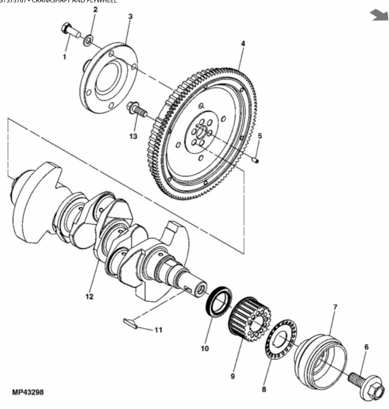
John Deere > Turf And Utility > UTILITY VEHICLE > XUV - UTILITY VEHICLE > XUV Gator Utility Vehicle 825i (Gas) > 20 ENGINE MM17029 > ST575767 - CRANKSHAFT AND FLYWHEEL
