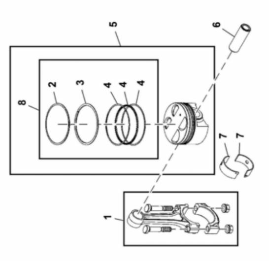
John Deere > Turf And Utility > UTILITY VEHICLE > XUV - UTILITY VEHICLE > XUV Gator Utility Vehicle 825i (Gas) > 20 ENGINE MM17029 > ST575766 - CONNECTING ROD AND PISTON
