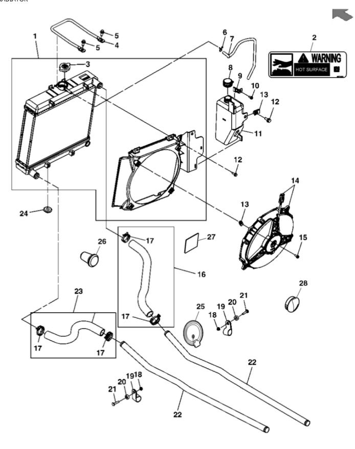
John Deere > Turf And Utility > UTILITY VEHICLE > XUV - UTILITY VEHICLE > XUV Gator Utility Vehicle 825i (Gas) > 20 ENGINE MM17029 > ST575773 - RADIATOR
