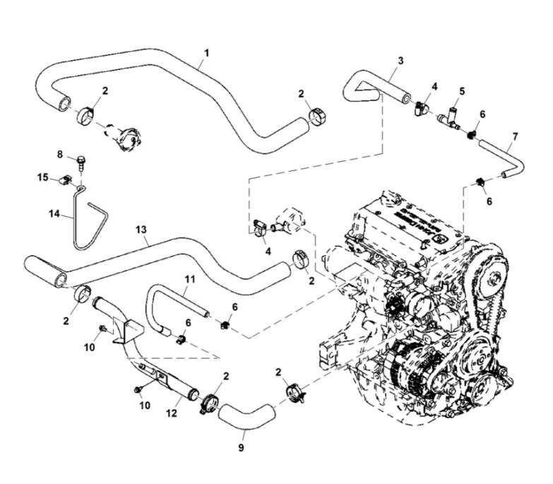
John Deere > Turf And Utility > UTILITY VEHICLE > XUV - UTILITY VEHICLE > XUV Gator Utility Vehicle 825i (Gas) > 20 ENGINE MM17029 > ST575774 - COOLANT LINES (-080000)
