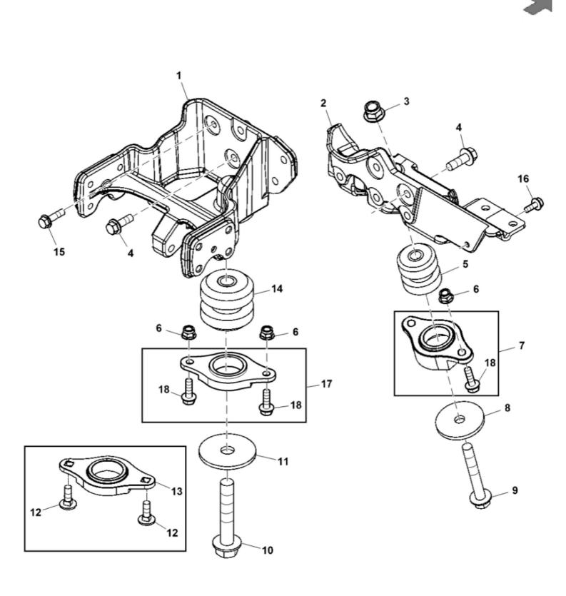
John Deere > Turf And Utility > UTILITY VEHICLE > XUV - UTILITY VEHICLE > XUV Gator Utility Vehicle 825i (Gas) > 20 ENGINE MM17029 > ST575775 - ISOLATOR
