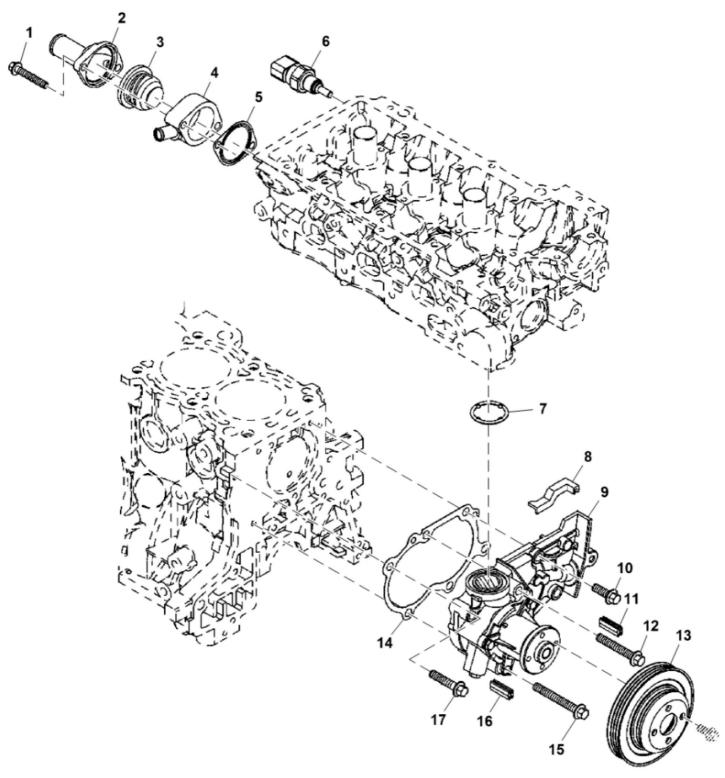
John Deere > Turf And Utility > UTILITY VEHICLE > XUV - UTILITY VEHICLE > XUV Gator Utility Vehicle 825i (Gas) > 20 ENGINE MM17029 > ST575772 - WATER PUMP AND THERMOSTAT
