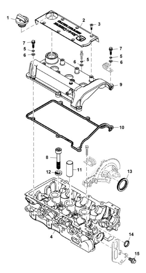
John Deere > Turf And Utility > UTILITY VEHICLE > XUV - UTILITY VEHICLE > XUV Gator Utility Vehicle 825i (Gas) > 20 ENGINE MM17029 > ST575770 - CYLINDER HEAD
