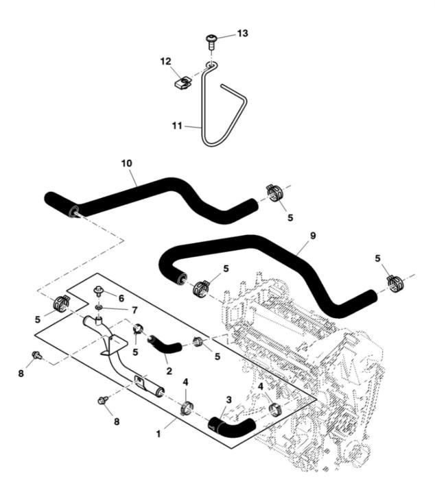
John Deere > Turf And Utility > UTILITY VEHICLE > XUV - UTILITY VEHICLE > XUV Gator Utility Vehicle 825i (Gas) > 20 ENGINE MM17029 > ST786761 - COOLANT LINES (080001 - )
