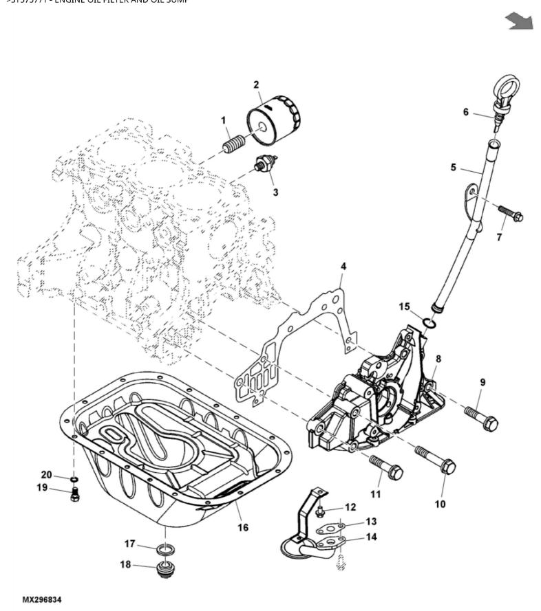
John Deere > Turf And Utility > UTILITY VEHICLE > XUV - UTILITY VEHICLE > XUV Gator Utility Vehicle 825i (Gas) > 20 ENGINE MM17029 > ST575771 - ENGINE OIL FILTER AND OIL SUMP
