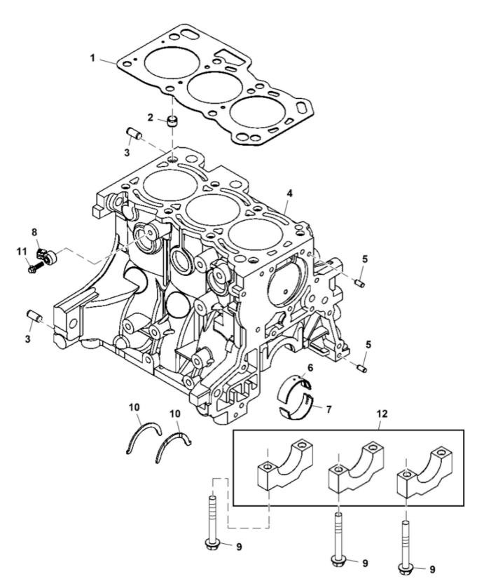
John Deere > Turf And Utility > UTILITY VEHICLE > XUV - UTILITY VEHICLE > XUV Gator Utility Vehicle 825i (Gas) > 20 ENGINE MM17029 > ST575765 - CYLINDER BLOCK
