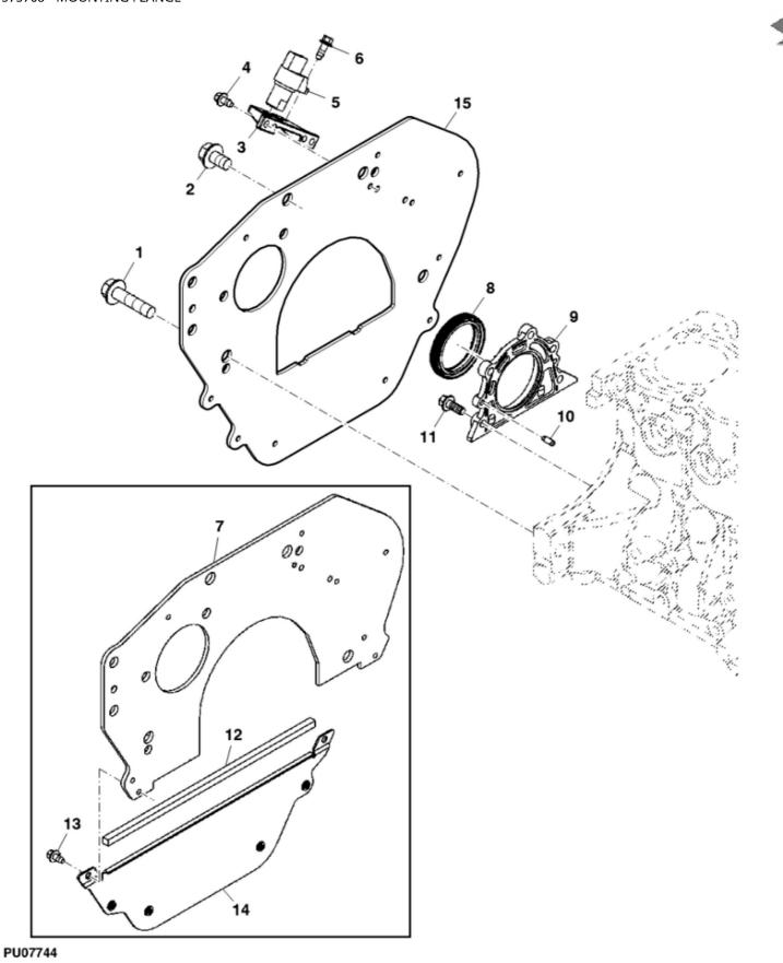
John Deere > Turf And Utility > UTILITY VEHICLE > XUV - UTILITY VEHICLE > XUV Gator Utility Vehicle 825i (Gas) > 20 ENGINE MM17029 > ST575768 - MOUNTING FLANGE
