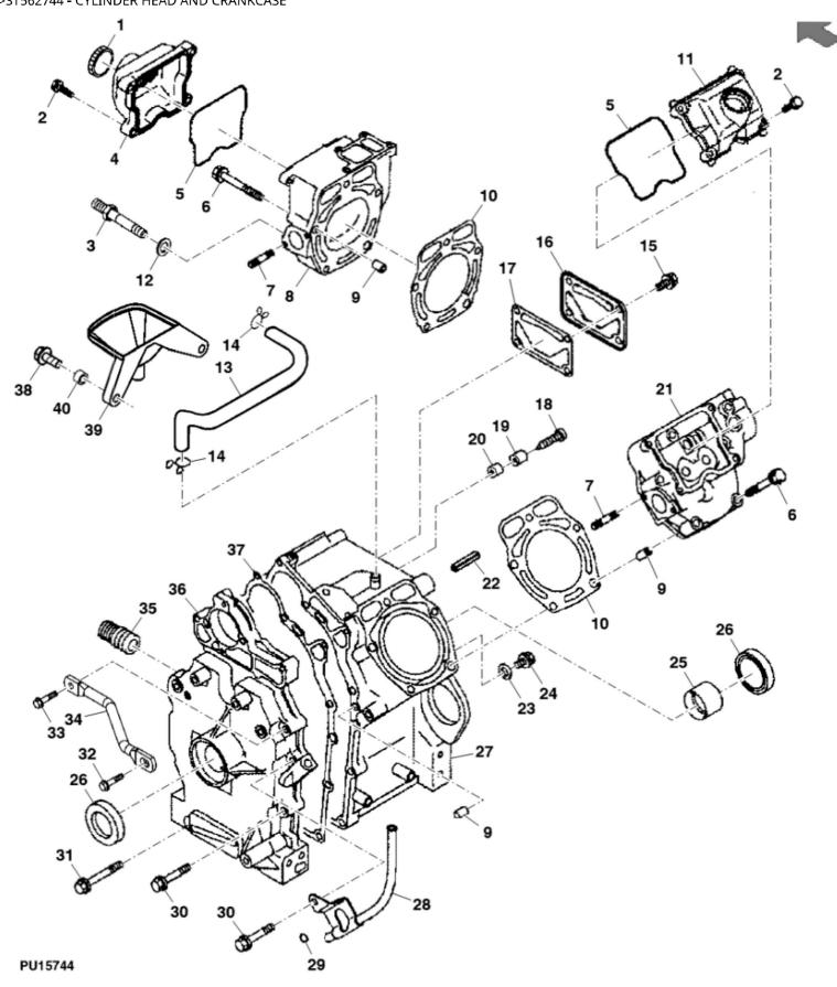
John Deere > Turf And Utility > UTILITY VEHICLE > XUV - UTILITY VEHICLE > XUV Gator Utility Vehicle 625i (Gas) > 20 ENGINE MM17590 > ST562744 - CYLINDER HEAD AND CRANKCASE
