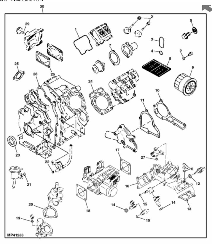
John Deere > Turf And Utility >UTILITY VEHICLE >XUV - UTILITY VEHICLE >XUV Gator Utility Vehicle 625i (Gas) >20 ENGINE MM17590 >ST562750 - ENGINE GASKET KIT
