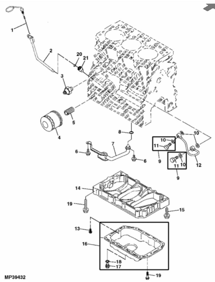
John Deere > Turf And Utility >UTILITY VEHICLE >XUV - UTILITY VEHICLE >XUV Gator Utility Vehicle 850D (Diesel) >20 ENGINE MM14374 >ST565141 - ENGINE OIL FILTER AND OIL SUMP
