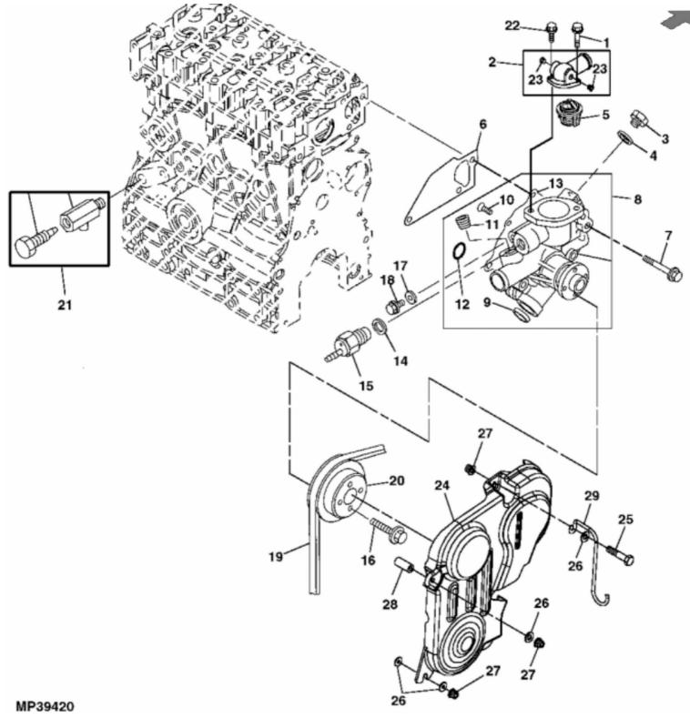
John Deere > Turf And Utility >UTILITY VEHICLE >XUV - UTILITY VEHICLE >XUV Gator Utility Vehicle 850D (Diesel) >20 ENGINE MM14374 >ST565143 - WATER PUMP AND THERMOSTAT
