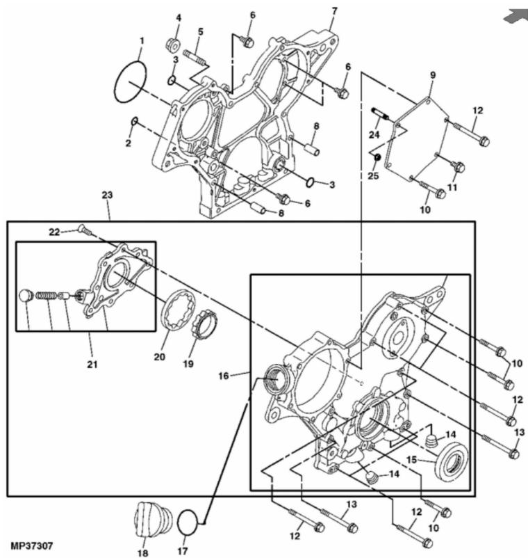
John Deere > Turf And Utility >UTILITY VEHICLE >XUV - UTILITY VEHICLE >XUV Gator Utility Vehicle 850D (Diesel) >20 ENGINE MM14374 >ST565142 - GEARCASE AND OIL PUMP
