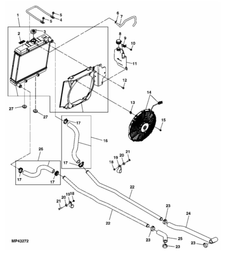
John Deere > Turf And Utility >UTILITY VEHICLE >XUV - UTILITY VEHICLE >XUV Gator Utility Vehicle 620i (Gas) >20 ENGINE MM14375 >ST565325 - RADIATOR (080001 - )
