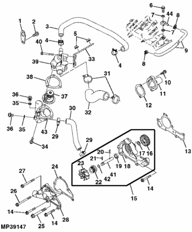
John Deere > Turf And Utility >UTILITY VEHICLE >XUV - UTILITY VEHICLE >XUV Gator Utility Vehicle 620i (Gas) >20 ENGINE MM14375 >ST565321 - WATER PUMP AND THERMOSTAT
