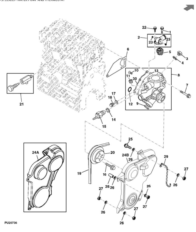
John Deere > Turf And Utility > UTILITY VEHICLE > TH - UTILITY VEHICLE > TH 6X4 Gator Utility Vehicle (Diesel) > 20 ENGINE MM17403 > ST559855 - WATER PUMP AND THERMOSTAT
