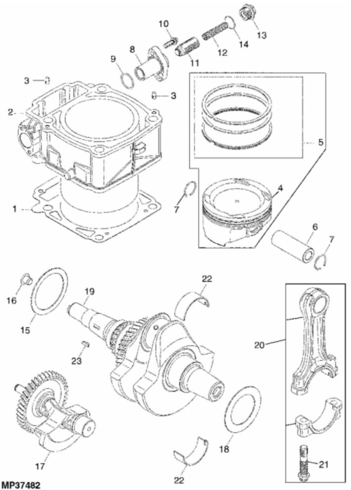
John Deere > Turf And Utility >UTILITY VEHICLE >UATV - UTILITY VEHICLE >Buck Auto Utility All Terrain Vehicle (UATV) Worldwide Edition >20 ENGINE AND POWER TRAIN >ST594664 - CRANKSHAFT AND PISTON ASSEMBLY
