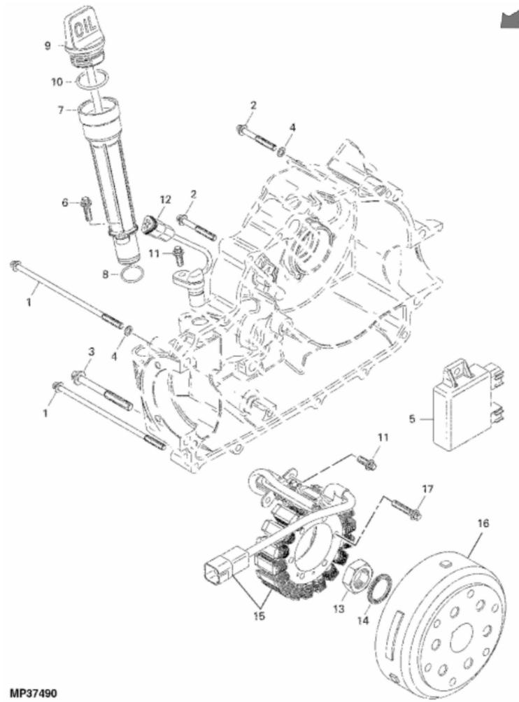
John Deere > Turf And Utility >UTILITY VEHICLE >UATV - UTILITY VEHICLE >Buck Auto Utility All Terrain Vehicle (UATV) Worldwide Edition >20 ENGINE AND POWER TRAIN >ST594666 - MAGNETO
