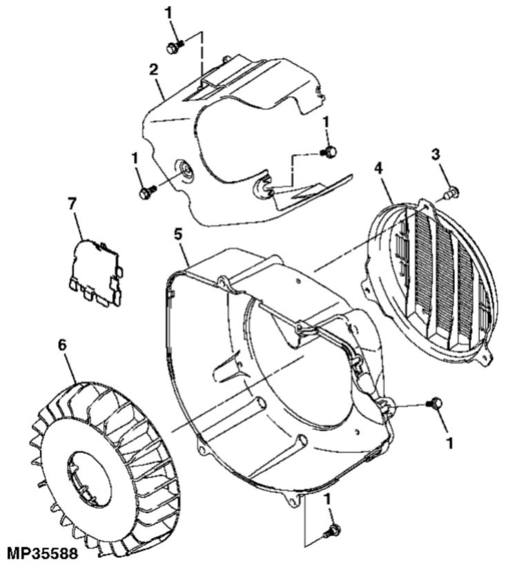
John Deere > Turf And Utility >UTILITY VEHICLE >TX - UTILITY VEHICLE >TX Turf or TX 4X2 Turf Gator Utility Vehicle >20 ENGINE >ST486622 - ENGINE BLOWER HOUSING
