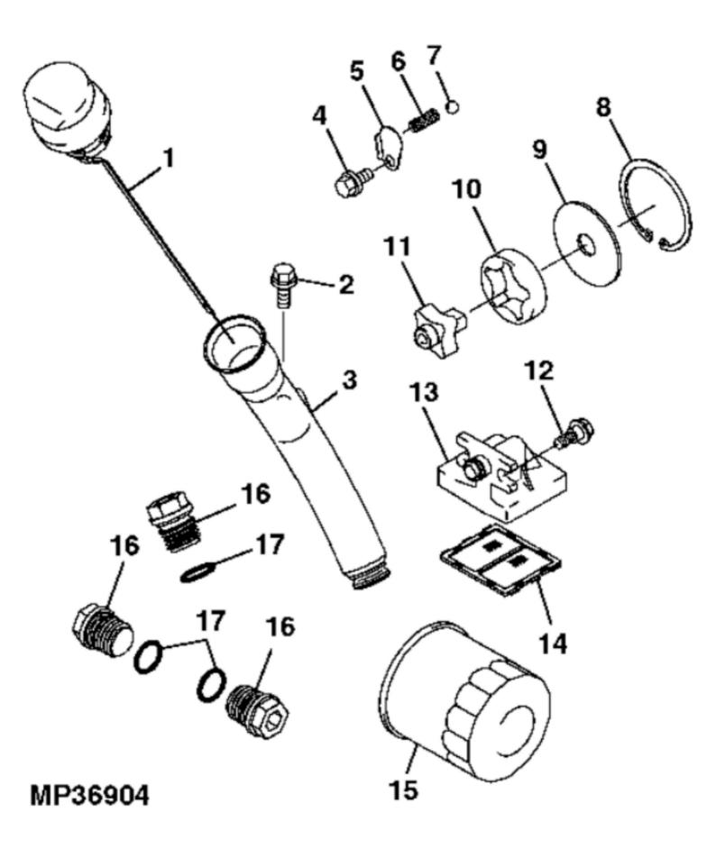
John Deere > Turf And Utility >UTILITY VEHICLE >TX - UTILITY VEHICLE >TX Turf or TX 4X2 Turf Gator Utility Vehicle >20 ENGINE >ST486621 - ENGINE OIL PUMP
