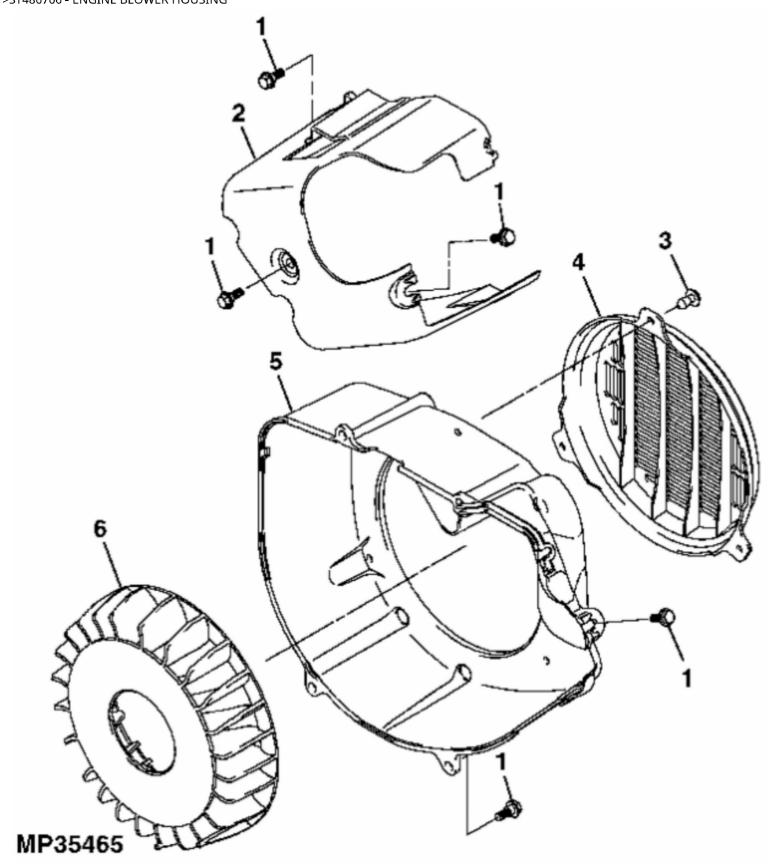
John Deere > Turf And Utility > UTILITY VEHICLE > TX - UTILITY VEHICLE > TX or TX 4X2 Gator Utility Vehicle > 20 ENGINE FJ400D MM17712 > ST486766 - ENGINE BLOWER HOUSING
