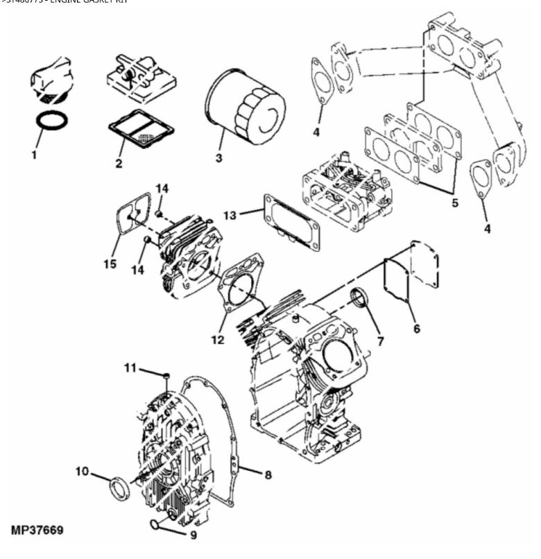
John Deere > Turf And Utility > UTILITY VEHICLE > TX - UTILITY VEHICLE > TX or TX 4X2 Gator Utility Vehicle > 21 ENGINE FH601D MM17636 > ST486775 - ENGINE GASKET KIT
