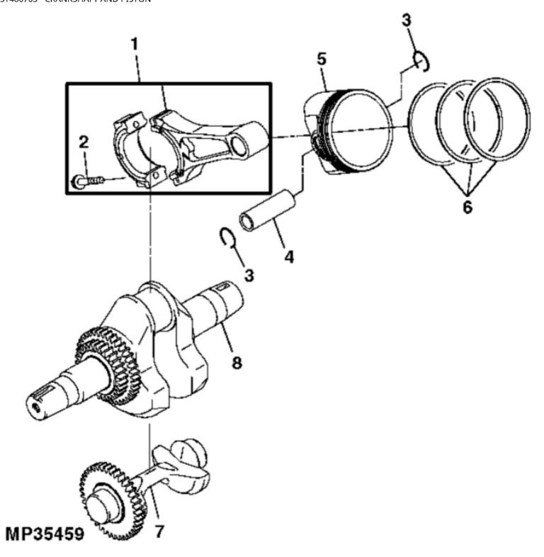
John Deere > Turf And Utility > UTILITY VEHICLE > TX - UTILITY VEHICLE > TX or TX 4X2 Gator Utility Vehicle > 20 ENGINE FJ400D MM17712 > ST486763 - CRANKSHAFT AND PISTON
