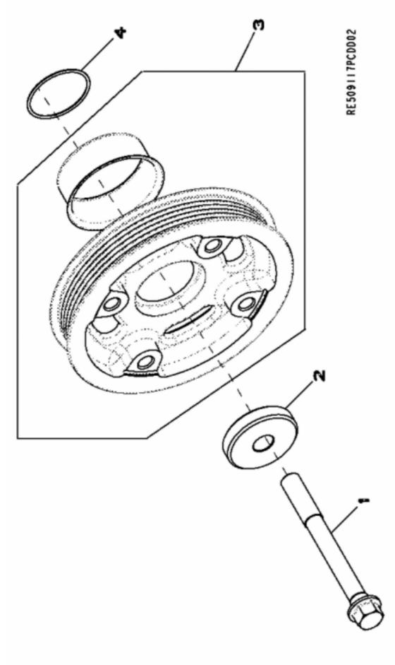
John Deere > Turf And Utility >TRACTOR, COMPACT UTILITY >4520 - TRACTOR, COMPACT UTILITY >4520 Compact Utility Tractor >20 ENGINE 4024TLV02-RE516054 >5T293043 - 1301 CRANKSHAFT PULLEY
