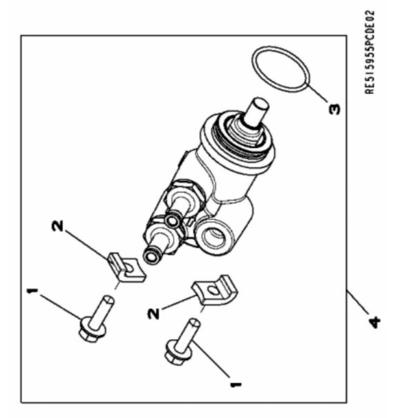
John Deere > Turf And Utility > TRACTOR, COMPACT UTILITY >4320 - TRACTOR, COMPACT UTILITY >4320 Compact Utility Tractor >20 ENGINE 4024TLV01-RE516053 > ST293059 - 3702 FUEL TRANSFER PUMP
