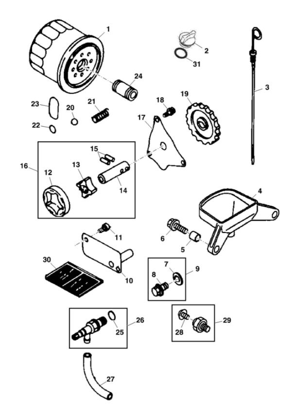
John Deere > Turf And Utility >UTILITY VEHICLE >X - UTILITY VEHICLE >4X2 HPX, 4X4 HPX AND 4X4 Trail HPX Gator Utility Vehicle (Gas) >20 ENGINE MM17625 >ST560052 - ENGINE OIL PUMP AND FILTER
