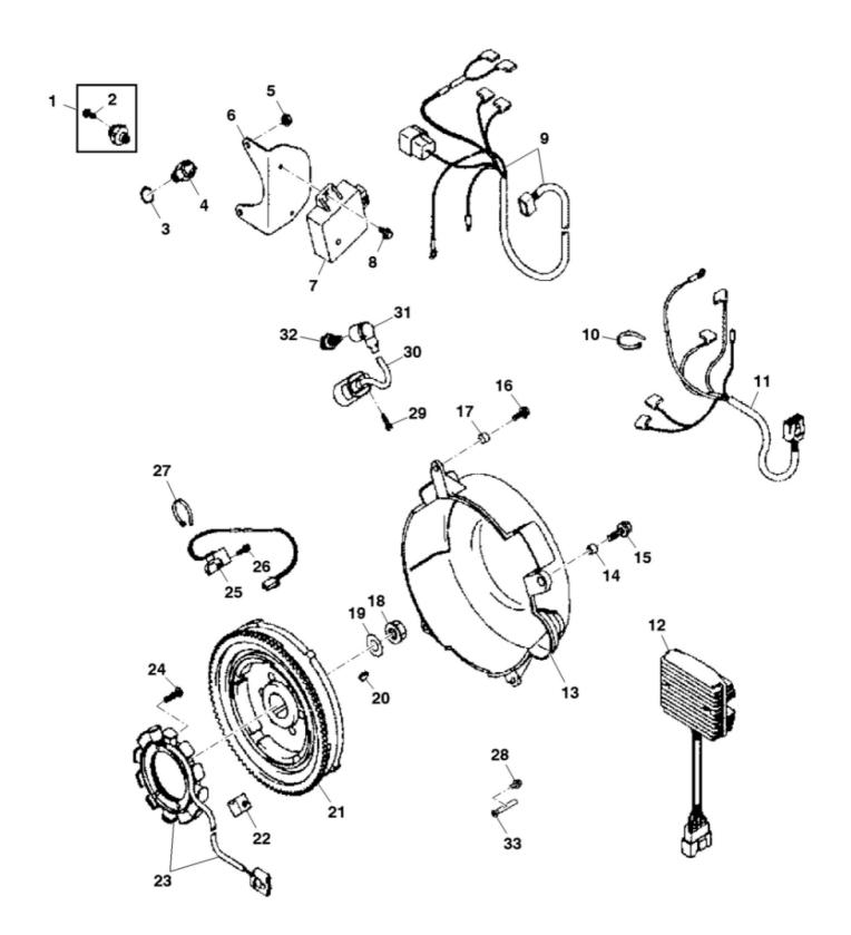
John Deere > Turf And Utility >UTILITY VEHICLE >X - UTILITY VEHICLE >4X2 HPX, 4X4 HPX AND 4X4 Trail HPX Gator Utility Vehicle (Gas) >20 ENGINE MM17625 >ST560054 - FLYWHEEL, IGNITION COIL AND STATOR
