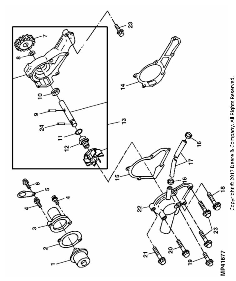
John Deere > Turf And Utility >UTILITY VEHICLE >X - UTILITY VEHICLE >4X2 HPX, 4X4 HPX AND 4X4 Trail HPX Gator Utility Vehicle (Gas) >20 ENGINE MM17625 >ST560053 - WATER PUMP AND THERMOSTAT
