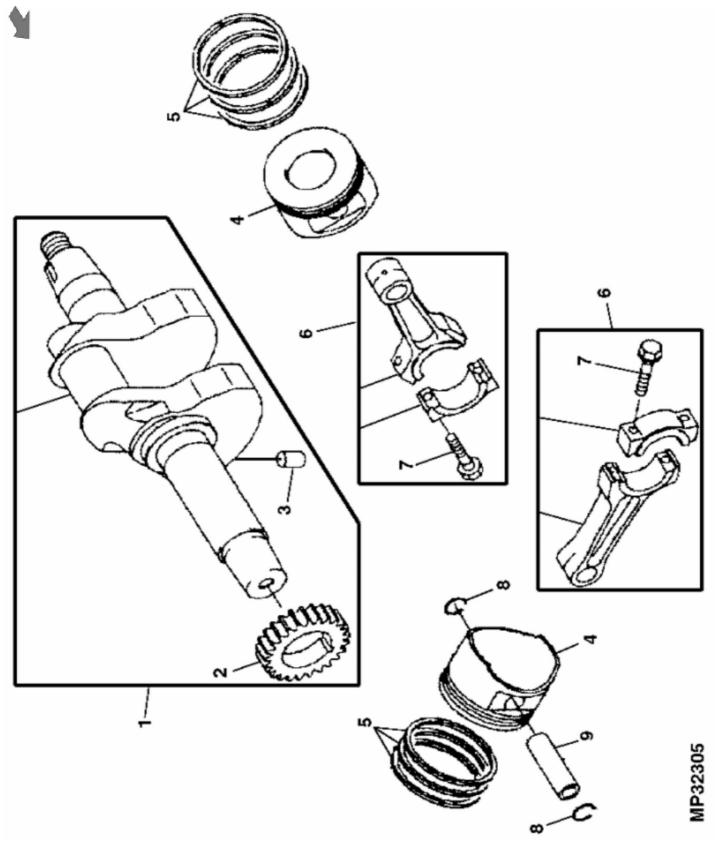
John Deere > Turf And Utility >UTILITY VEHICLE >X - UTILITY VEHICLE >4X2 HPX, 4X4 HPX AND 4X4 Trail HPX Gator Utility Vehicle (Gas) >20 ENGINE MM17625 >ST560049 - CRANKSHAFT AND PISTON ASSEMBLY
