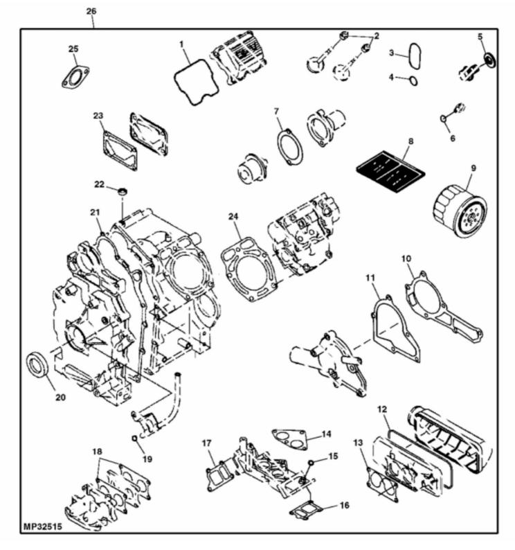
John Deere > Turf And Utility >UTILITY VEHICLE >X - UTILITY VEHICLE >4X2 HPX, 4X4 HPX AND 4X4 Trail HPX Gator Utility Vehicle (Gas) >20 ENGINE MM17625 >ST560055 - ENGINE GASKET KIT
