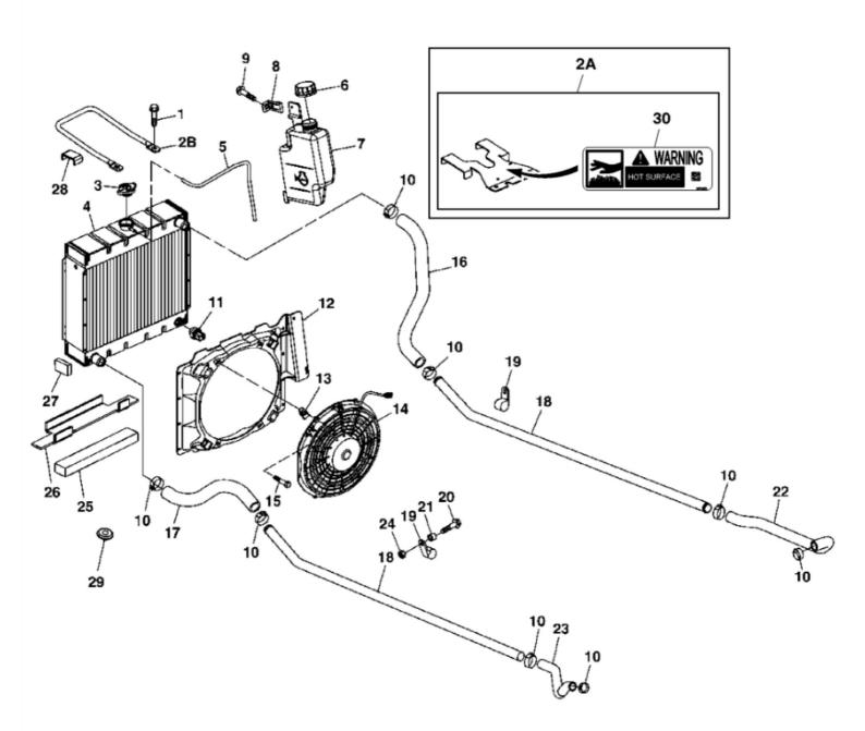
John Deere > Turf And Utility >UTILITY VEHICLE >X - UTILITY VEHICLE >4X2 HPX, 4X4 HPX AND 4X4 Trail HPX Gator Utility Vehicle (Gas) >20 ENGINE MM17625 >ST560056 - RADIATOR ( - 090000)
