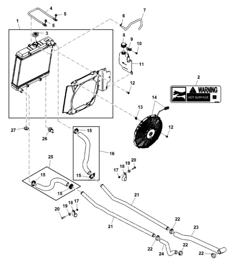
John Deere > Turf And Utility >UTILITY VEHICLE >X - UTILITY VEHICLE >4X2 HPX, 4X4 HPX AND 4X4 Trail HPX Gator Utility Vehicle (Gas) >20 ENGINE MM17625 >ST560057 - RADIATOR (090001 - )
