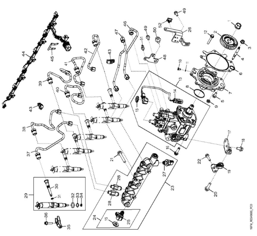
John Deere > Turf And Utility >TRACTOR >6155RH - TRACTOR >6155R, 6155RH Tractor (North America Edition, Engine SN: 6068UXXXXXX)(Final Tier 4) >E1 ENGINE 6068RW429-DZ100119-ETN126468 >E100 ENGINE 6068RW429-DZ100119-ETN126468 6068RW429 >ST751293 - 16FM FUEL INJECTION SYSTEM
