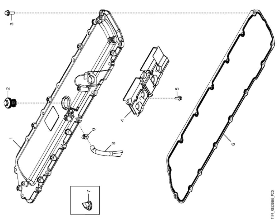
John Deere > Turf And Utility >TRACTOR >6155RH - TRACTOR >6155R, 6155RH Tractor (North America Edition, Engine SN: 6068UXXXXXX)(Final Tier 4) >E1 ENGINE 6068RW429-DZ100119-ETN126468 >E100 ENGINE 6068RW429-DZ100119-ETN126468 6068RW429 >ST164694 - 1174 ROCKER ARM COVER
