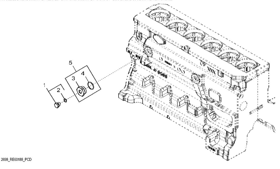
John Deere > Turf And Utility >TRACTOR >6215R - TRACTOR >6215R Tractor (North America Edition, Engine SN: 6068UXXXXXX)(Final Tier 4) >E1 DIESEL ENGINE 6068RW424-RE567257-ETN115183 6068RW424 >ST348491 - 2698 ENGINE COOLANT HEATER FITTINGS
