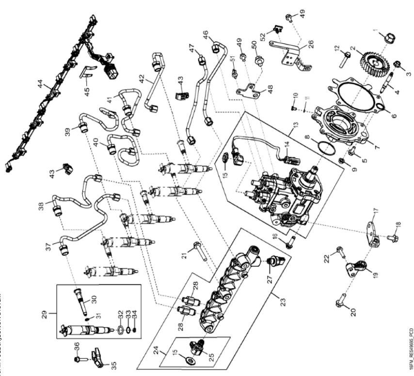
John Deere > Turf And Utility >TRACTOR >6215R - TRACTOR >6215R Tractor (North America Edition, Engine SN: 6068UXXXXXXX)(Final Tier 4) >E1 DIESEL ENGINE 6068RW424-RE567257-ETN115183 6068RW424 >ST751293 - 16FM FUEL INJECTION SYSTEM
