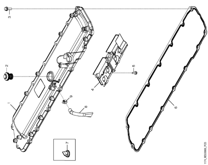
John Deere > Turf And Utility >TRACTOR >6215R - TRACTOR >6215R Tractor (North America Edition, Engine SN: 6068UXXXXXX)(Final Tier 4) >E1 DIESEL ENGINE 6068RW424-RE567257-ETN115183 6068RW424 >ST164694 - 1174 ROCKER ARM COVER
