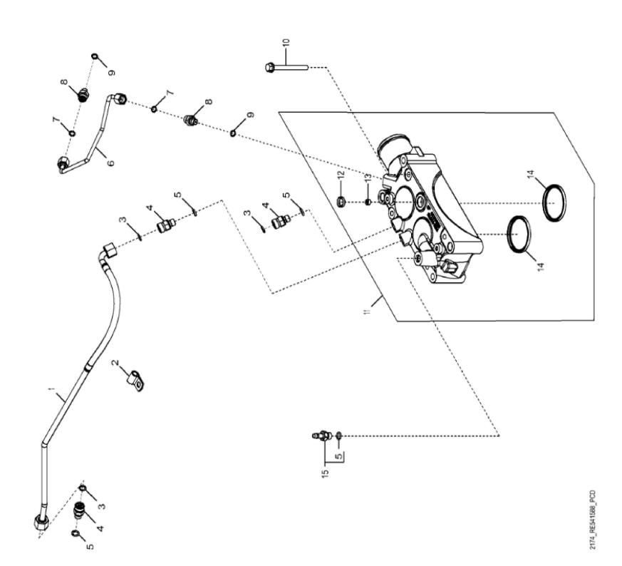
John Deere > Turf And Utility >TRACTOR >6195R - TRACTOR >6195R Tractor (North America Edition, Engine SN: 6068UXXXXXXX)(Final Tier 4) >E1 DIESEL ENGINE 6068RW424-RE567257-ETN115183 6068RW424 >ST261980 - 2174 THERMOSTAT COVER
