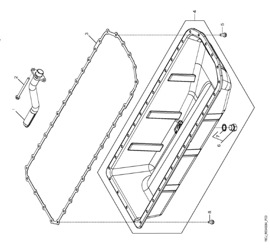
John Deere > Turf And Utility >TRACTOR >6195R - TRACTOR >6195R Tractor (Europe Edition, Engine SN: 6068UXXXXXXX)(Final Tier 4) >E1 ENGINE 6068HL501-DD22296-ETN111219 6068HL501 >ST330886 - 19CJ OIL PAN
