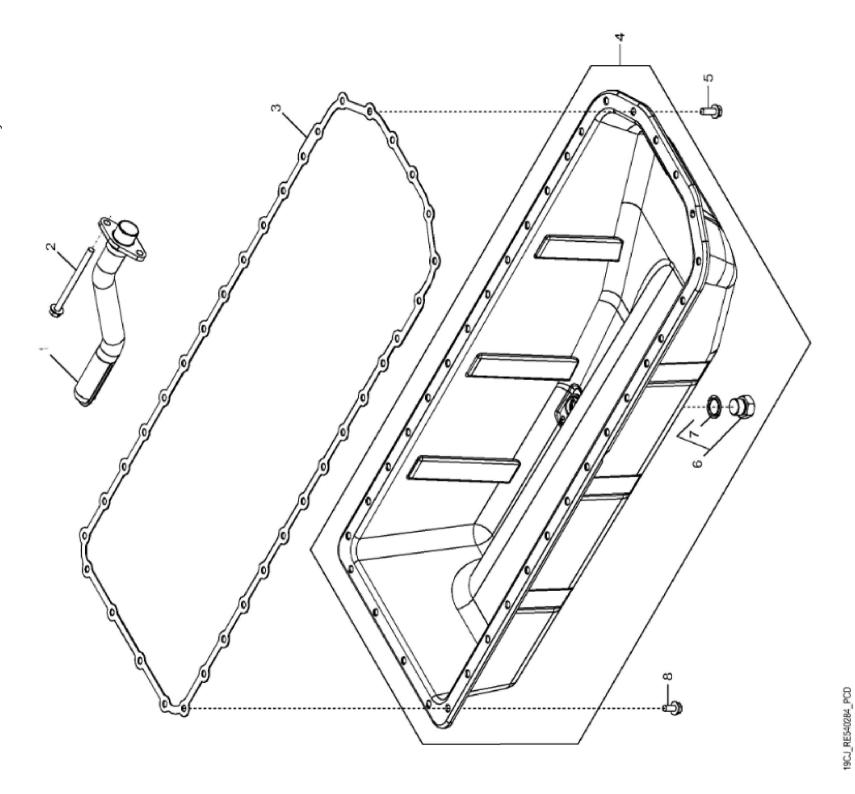
John Deere > Turf And Utility >TRACTOR >6175R - TRACTOR >6175R Tractor (Europe Edition, Engine SN: 6068UXXXXXXX)(Final Tier 4) >E1 ENGINE 6068HL499-DD22295-ETN111220 >E100 ENGINE 6068HL499-DD22295-ETN111220 6068HL499 >ST330886 - 19CJ OIL PAN
