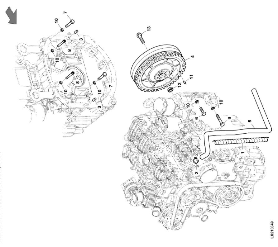
John Deere > Turf And Utility > TRACTOR > F5AE9454H - TRACTOR > 5075GV Tractor (Engine F5A) T3A (Europe Edition) > 20 ENGINE > ST798602 - FLYWHEEL / MOUNTING PARTS, ENGINE
