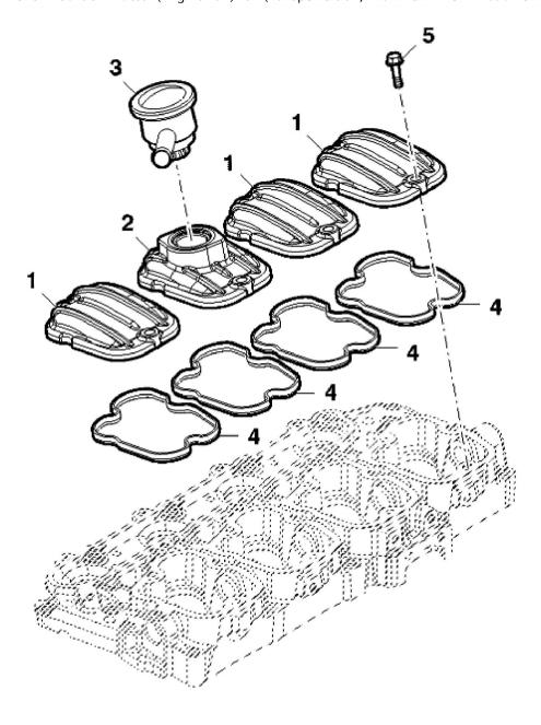
John Deere > Turf And Utility >TRACTOR >F5AE9454H - TRACTOR >5075GV Tractor (Engine F5A) T3A (Europe Edition) >20 ENGINE >ST774096 - CYLINDER HEAD COVER
