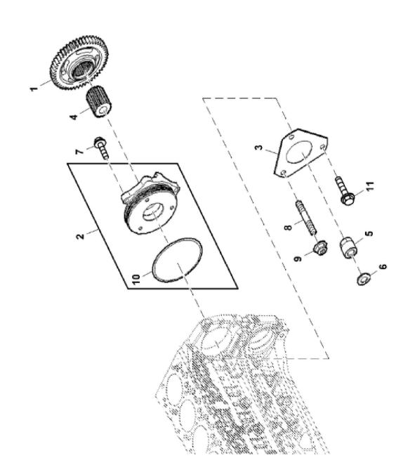
John Deere > Turf And Utility >TRACTOR >F4CE9484F - TRACTOR >5100GN Tractor (Engine F4C) T3A (Europe Edition) >20 ENGINE >ST810274 - DRIVE, FUEL INJECTION PUMP
