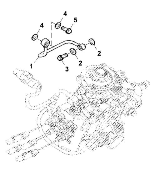
John Deere > Turf And Utility >TRACTOR >F4CE9484F - TRACTOR >5100GN Tractor (Engine F4C) T3A (Europe Edition) >20 ENGINE >ST810276 - TUBE, FUEL INJECTION PUMP
