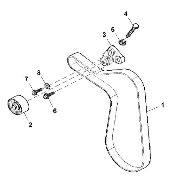
John Deere > Turf And Utility >TRACTOR >F4CE9484F - TRACTOR >5100GN Tractor (Engine F4C) T3A (Europe Edition) >20 ENGINE >ST810175 - DRIVE BELT / PULLEY
