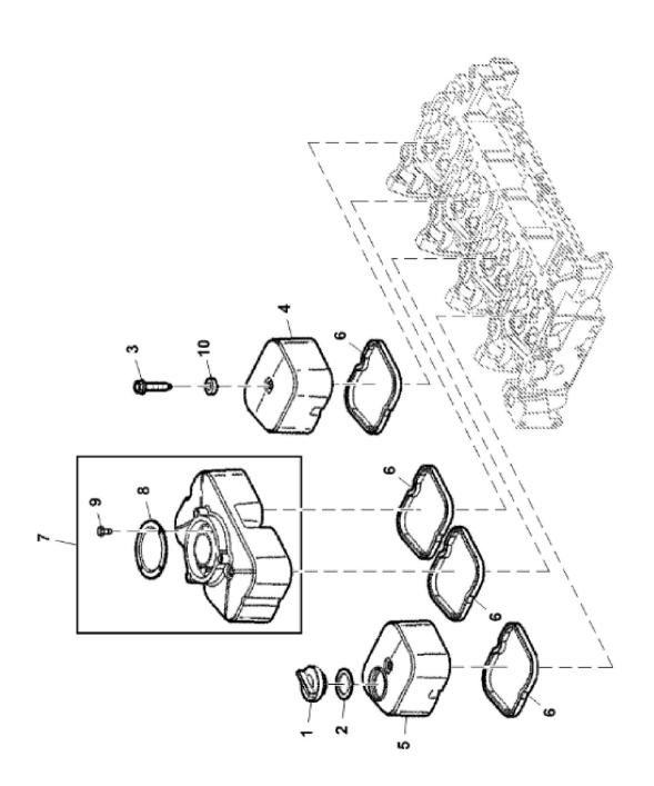
John Deere > Turf And Utility >TRACTOR >F4CE9484F - TRACTOR >5100GN Tractor (Engine F4C) T3A (Europe Edition) >20 ENGINE >ST810003 - CYLINDER HEAD COVER
