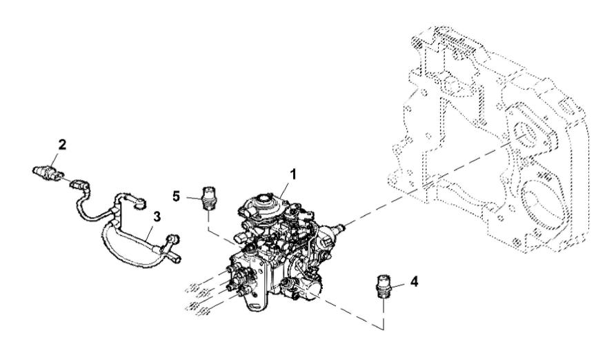
John Deere > Turf And Utility >TRACTOR >F4CE9484F - TRACTOR >5100GN Tractor (Engine F4C) T3A (Europe Edition) >20 ENGINE >ST810272 - FUEL INJECTION PUMP
