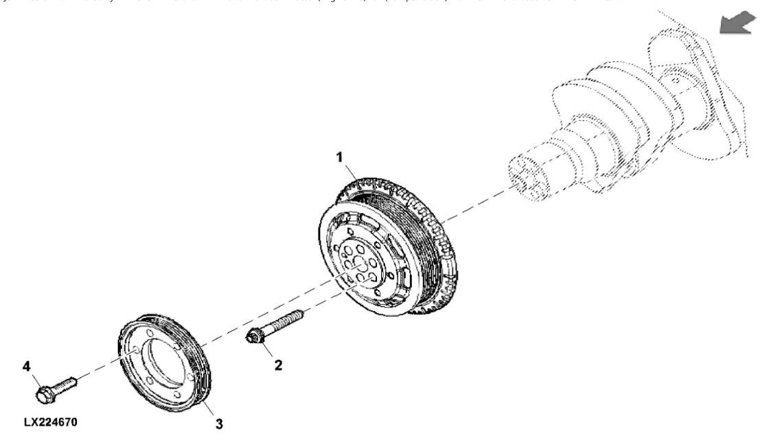
John Deere > Turf And Utility >TRACTOR >F4CE9484F - TRACTOR >5100GN Tractor (Engine F4C) T3A (Europe Edition) >20 ENGINE >ST810335 - CRANKSHAFT PULLEY
