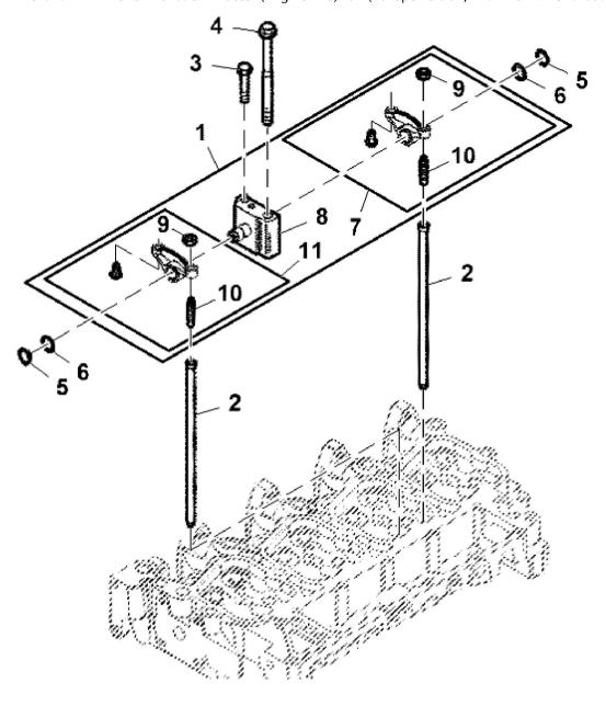
John Deere > Turf And Utility > TRACTOR > F4CE9484F - TRACTOR > 5100GN Tractor (Engine F4C) T3A (Europe Edition) > 20 ENGINE > ST810081 - ROCKER ARM / SHAFT
