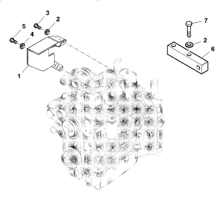
John Deere > Turf And Utility >TRACTOR >F4CE9484F - TRACTOR >5100GN Tractor (Engine F4C) T3A (Europe Edition) >20 ENGINE >ST798553 - MOUNTING PARTS, ENGINE
