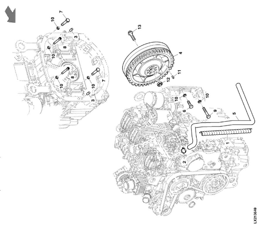
John Deere > Turf And Utility > TRACTOR > F5AE9484G - TRACTOR > 5085GN Tractor (Engine F5A) T3A (Europe Edition) > 20 ENGINE > ST798602 - FLYWHEEL / MOUNTING PARTS, ENGINE
