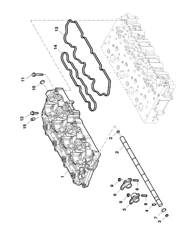
John Deere > Turf And Utility > TRACTOR > F5AE9454H - TRACTOR > 5075GN Tractor (Engine F5A) T3A (Europe Edition) > 20 ENGINE > ST774077 - CYLINDER HEAD HOUSING
