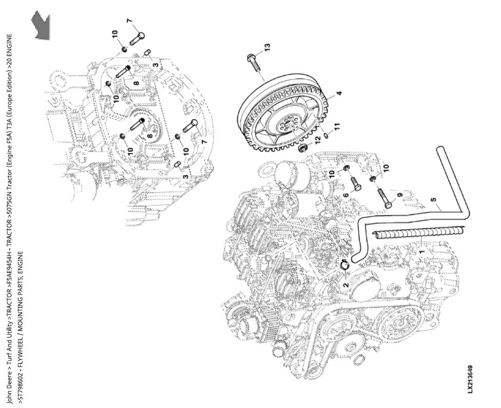
John Deere > Turf And Utility > TRACTOR > F5AE9454H - TRACTOR > 5075GN Tractor (Engine F5A) T3A (Europe Edition) > 20 ENGINE > ST798602 - FLYWHEEL / MOUNTING PARTS, ENGINE
