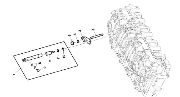
John Deere > Turf And Utility >TRACTOR >F5AE9454H - TRACTOR >5075GN Tractor (Engine F5A) T3A (Europe Edition) >20 ENGINE >ST776343 - INJECTION NOZZLE
