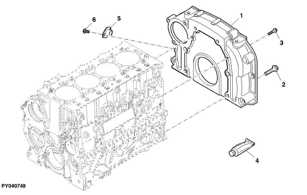
John Deere > Turf And Utility >TRACTOR >F5AE9454H - TRACTOR >5075GN Tractor (Engine F5A) T3A (Europe Edition) >20 ENGINE >ST776845 - FLYWHEEL HOUSING
