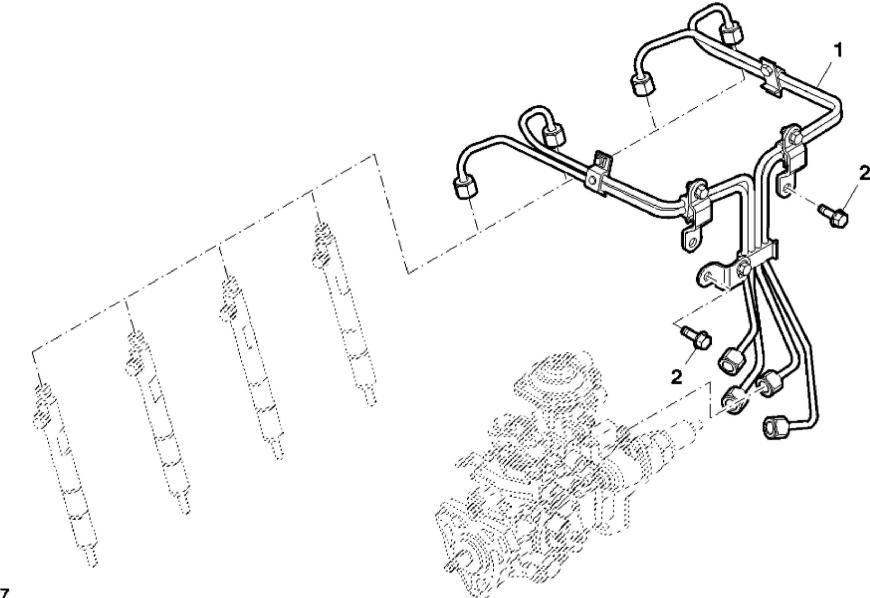
John Deere > Turf And Utility >TRACTOR >F5AE9454H - TRACTOR >5075GN Tractor (Engine F5A) T3A (Europe Edition) >20 ENGINE >ST774367 - FUEL LINES
