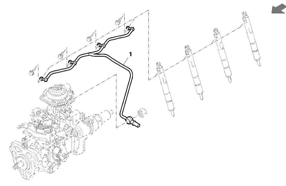
John Deere > Turf And Utility >TRACTOR >F5AE9454H - TRACTOR >5075GN Tractor (Engine F5A) T3A (Europe Edition) >20 ENGINE >ST774371 - FUEL LINES
