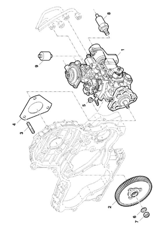
John Deere > Turf And Utility > TRACTOR > F5AE9454H - TRACTOR > 5075GN Tractor (Engine F5A) T3A (Europe Edition) > 20 ENGINE > ST810167 - FUEL INJECTION PUMP
