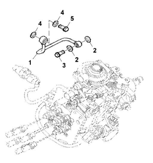
John Deere > Turf And Utility >TRACTOR >F4CE9484F - TRACTOR >5100GF Tractor (Engine F4C) T3A (Europe Edition) >20 ENGINE >ST810276 - TUBE, FUEL INJECTION PUMP
