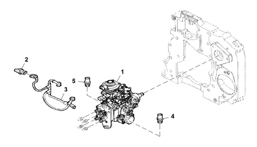
John Deere > Turf And Utility >TRACTOR >F4CE9484F - TRACTOR >5100GF Tractor (Engine F4C) T3A (Europe Edition) >20 ENGINE >ST810272 - FUEL INJECTION PUMP
