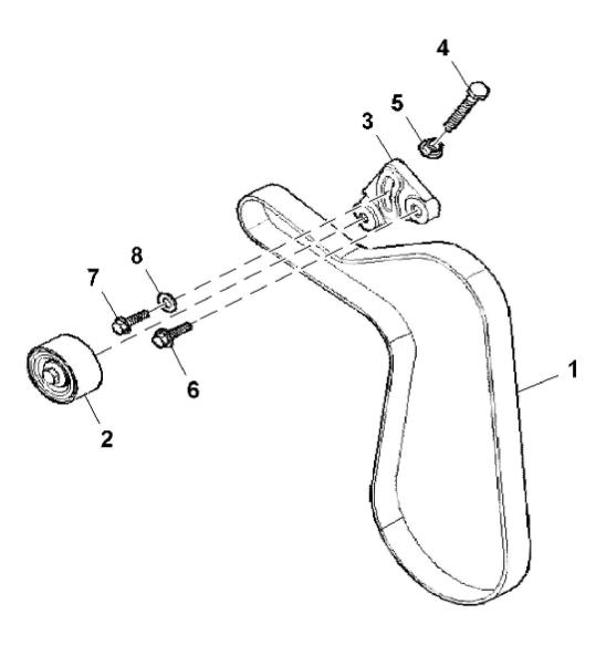
John Deere > Turf And Utility >TRACTOR >F4CE9484F - TRACTOR >5100GF Tractor (Engine F4C) T3A (Europe Edition) >20 ENGINE >ST810175 - DRIVE BELT / PULLEY
