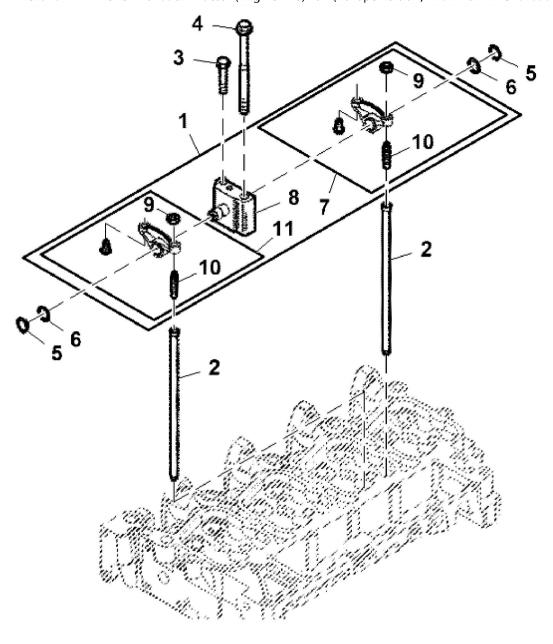
John Deere > Turf And Utility >TRACTOR >F4CE9484F - TRACTOR >5100GF Tractor (Engine F4C) T3A (Europe Edition) >20 ENGINE >ST810081 - ROCKER ARM / SHAFT
