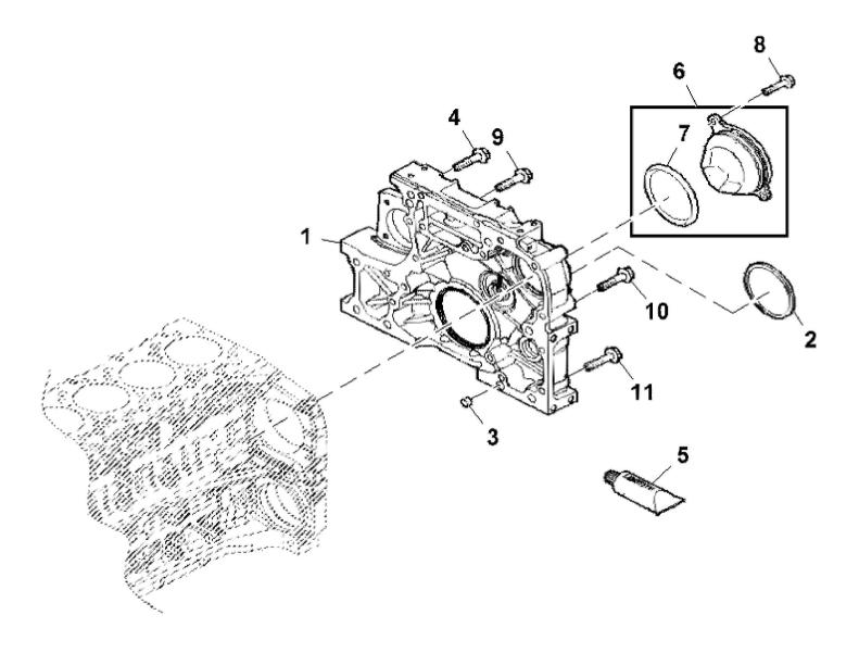
John Deere > Turf And Utility > TRACTOR > F4CE9484F - TRACTOR > 5100GF Tractor (Engine F4C) T3A (Europe Edition) > 20 ENGINE > ST810155 - FLYWHEEL HOUSING
