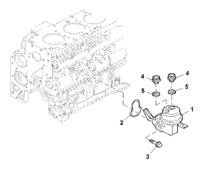
John Deere > Turf And Utility >TRACTOR >F4CE9484F - TRACTOR >5100GF Tractor (Engine F4C) T3A (Europe Edition) >20 ENGINE >ST810073 - FUEL PUMP
