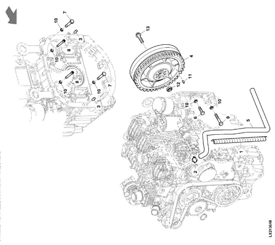
John Deere > Turf And Utility >TRACTOR >F5AE9484G - TRACTOR >5085GF Tractor (Engine F5A) T3A (Europe Edition) >20 ENGINE >ST798602 - FLYWHEEL / MOUNTING PARTS, ENGINE
