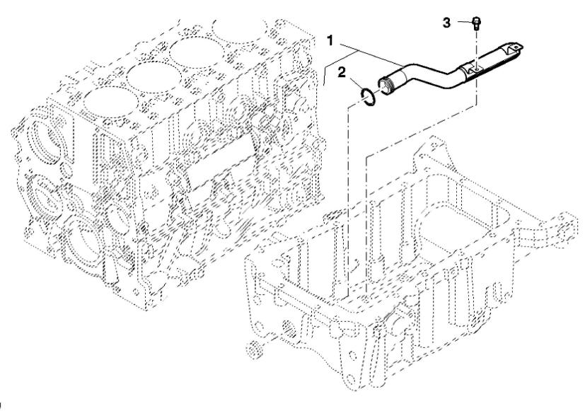
John Deere > Turf And Utility >TRACTOR >F5AE9454H - TRACTOR >5075GF Tractor (Engine F5A) T3A (Europe Edition) >20 ENGINE >ST774119 - SUCTION HOSE
