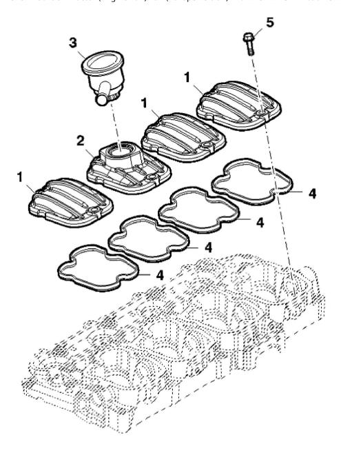
John Deere > Turf And Utility >TRACTOR >F5AE9454H - TRACTOR >5075GF Tractor (Engine F5A) T3A (Europe Edition) >20 ENGINE >ST774096 - CYLINDER HEAD COVER
