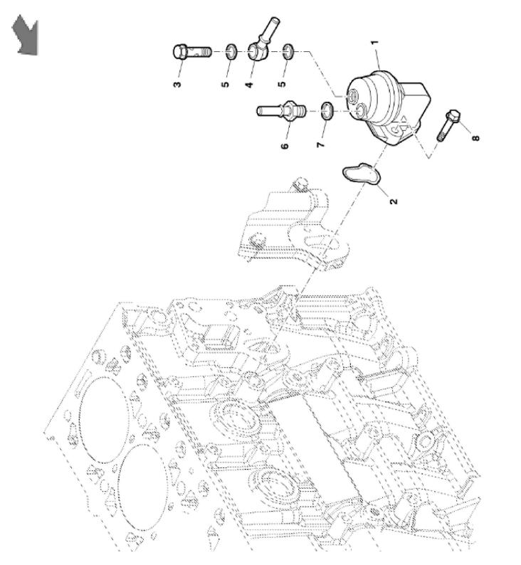
John Deere > Turf And Utility >TRACTOR >F5AE9454H - TRACTOR >5075GF Tractor (Engine F5A) T3A (Europe Edition) >20 ENGINE >ST774360 - FUEL PUMP
