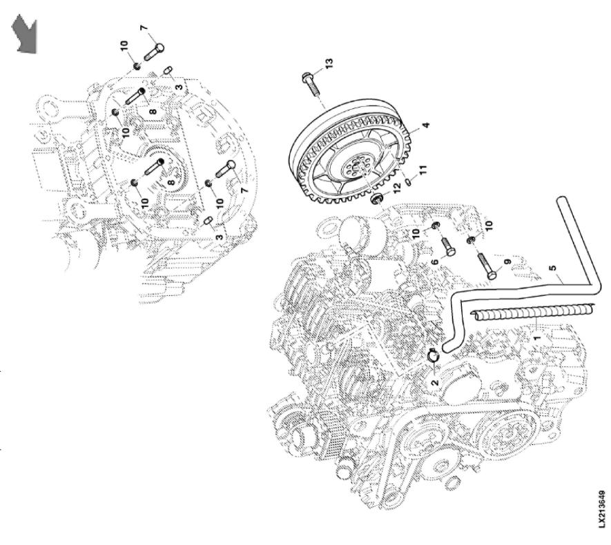
John Deere > Turf And Utility >TRACTOR >F5AE9454H - TRACTOR >5075GF Tractor (Engine F5A) T3A (Europe Edition) >20 ENGINE >ST798602 - FLYWHEEL / MOUNTING PARTS, ENGINE
