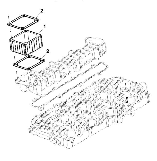
John Deere > Turf And Utility >TRACTOR >F5AE9454H - TRACTOR >5075GF Tractor (Engine F5A) T3A (Europe Edition) >20 ENGINE >ST774894 - SPACER, INTAKE MANIFOLD
