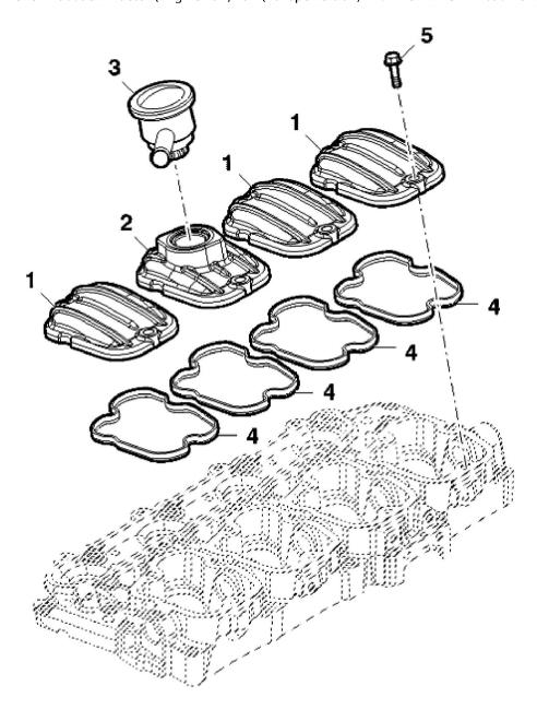
John Deere > Turf And Utility >TRACTOR >F5AE9484G - TRACTOR >5085GL Tractor (Engine F5A) T3A (Europe Edition) >20 ENGINE >ST774096 - CYLINDER HEAD COVER
