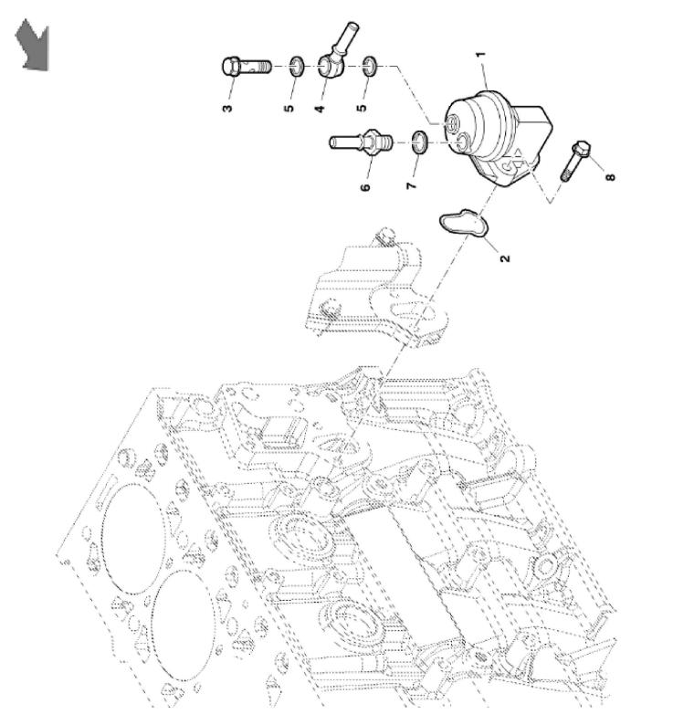
John Deere > Turf And Utility >TRACTOR >F5AE9484G - TRACTOR >5085GL Tractor (Engine F5A) T3A (Europe Edition) >20 ENGINE >ST774360 - FUEL PUMP
