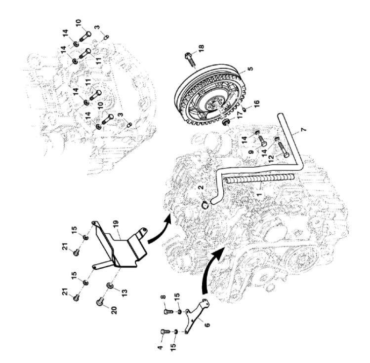
John Deere > Turf And Utility >TRACTOR >F5AE9484G - TRACTOR >5085GL Tractor (Engine F5A) T3A (Europe Edition) >20 ENGINE >ST783718 - MOUNTING PARTS, ENGINE / FLYWHEEL
