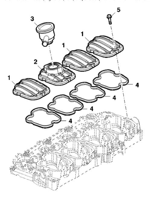
John Deere > Turf And Utility >TRACTOR >F5AE9484B - TRACTOR >5075GL Tractor (Engine F5A) T3A (Europe Edition) >20 ENGINE >ST774096 - CYLINDER HEAD COVER
