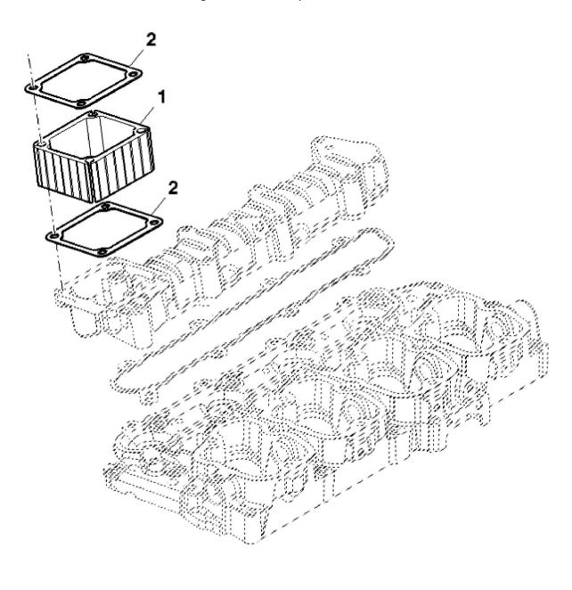
John Deere > Turf And Utility >TRACTOR >F5AE9484B - TRACTOR >5075GL Tractor (Engine F5A) T3A (Europe Edition) >20 ENGINE >ST774894 - SPACER, INTAKE MANIFOLD
