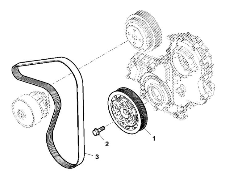
John Deere > Turf And Utility >TRACTOR >F5AE9484B - TRACTOR >5075GL Tractor (Engine F5A) T3A (Europe Edition) >20 ENGINE >ST774085 - DRIVE BELT / PULLEY
