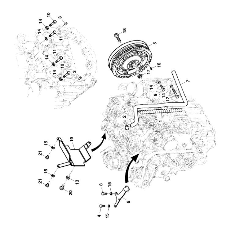
John Deere > Turf And Utility >TRACTOR >F5AE9484B - TRACTOR >5075GL Tractor (Engine F5A) T3A (Europe Edition) >20 ENGINE >ST783718 - MOUNTING PARTS, ENGINE / FLYWHEEL
