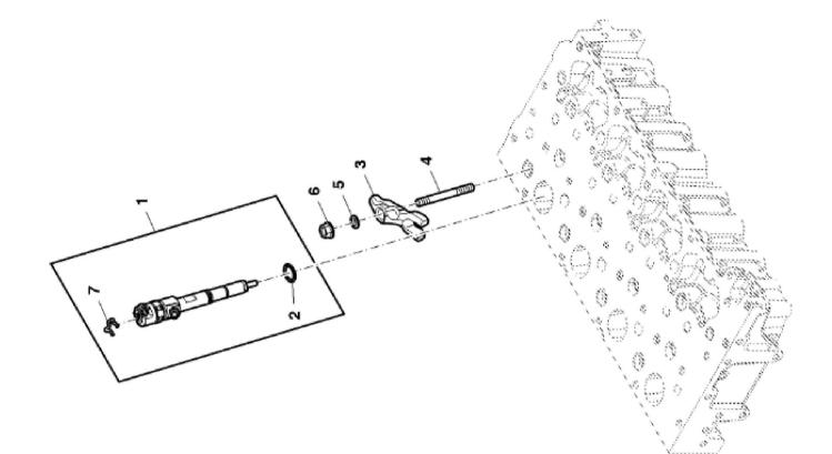
John Deere > Turf And Utility >TRACTOR >F5DFL413T - TRACTOR >5090GH Tractor (Engine F5D) IT4 (Europe Edition) >20 ENGINE >ST776357 - INJECTION NOZZLE
