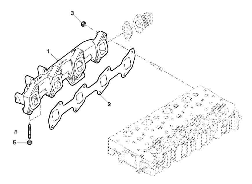
John Deere > Turf And Utility >TRACTOR >F5DFL413T - TRACTOR >5090GH Tractor (Engine F5D) IT4 (Europe Edition) >20 ENGINE >ST793021 - EXHAUST MANIFOLD
