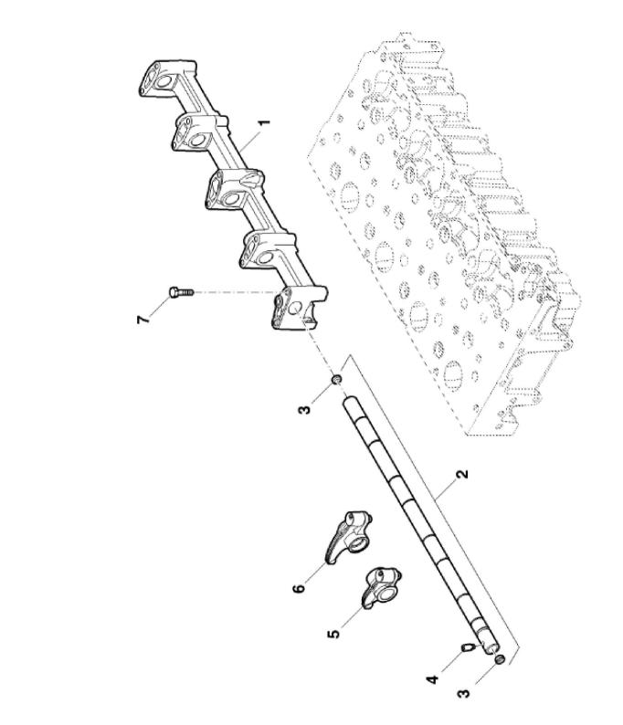
John Deere > Turf And Utility >TRACTOR >F5DFL413T - TRACTOR >5090GH Tractor (Engine F5D) IT4 (Europe Edition) >20 ENGINE >ST775005 - ROCKER ARM / SHAFT
