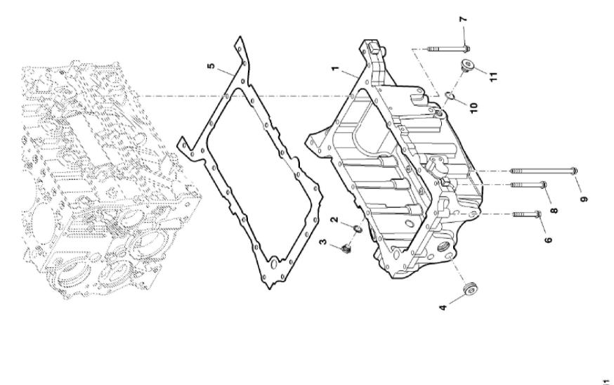
John Deere > Turf And Utility >TRACTOR >F5DFL413T - TRACTOR >5090GH Tractor (Engine F5D) IT4 (Europe Edition) >20 ENGINE >ST788768 - OIL PAN
