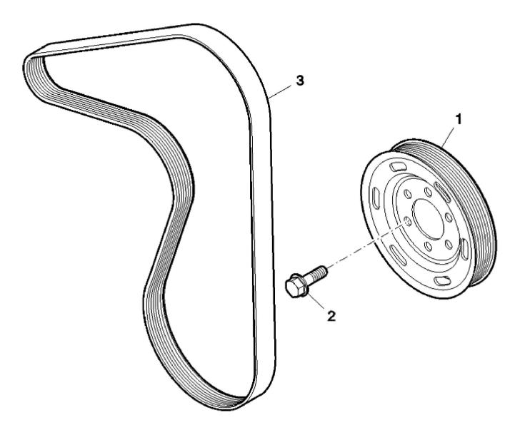
John Deere > Turf And Utility >TRACTOR >F5DFL413T - TRACTOR >5090G Tractor (Engine F5D) IT4 (Europe Edition) >20 ENGINE >ST774090 - DRIVE BELT / PULLEY
