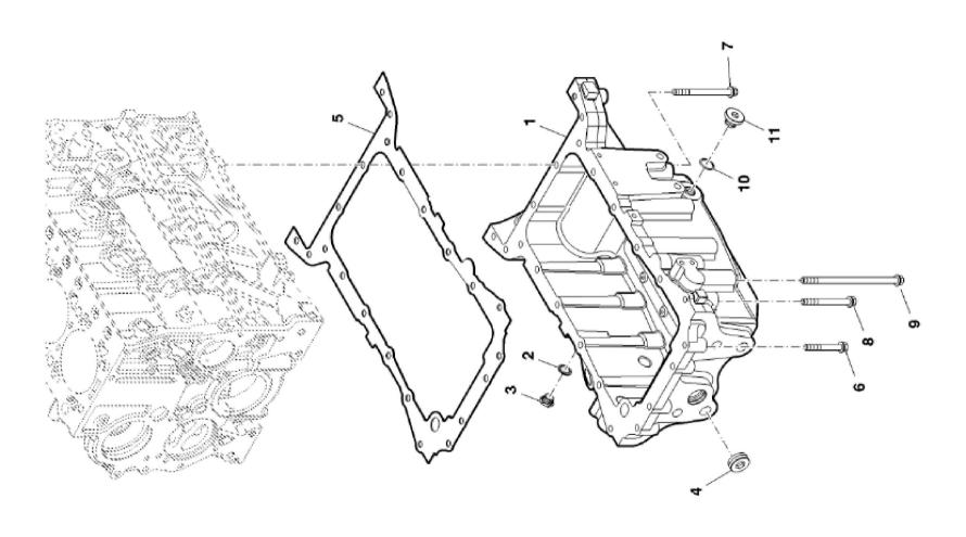
John Deere > Turf And Utility >TRACTOR >F5DFL413T - TRACTOR >5090G Tractor (Engine F5D) IT4 (Europe Edition) >20 ENGINE >ST788768 - OIL PAN
