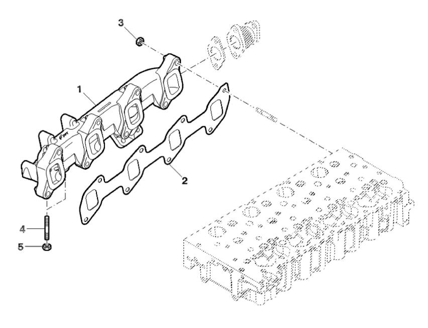
John Deere > Turf And Utility >TRACTOR >F5DFL413T - TRACTOR >5090G Tractor (Engine F5D) IT4 (Europe Edition) >20 ENGINE >ST793021 - EXHAUST MANIFOLD
