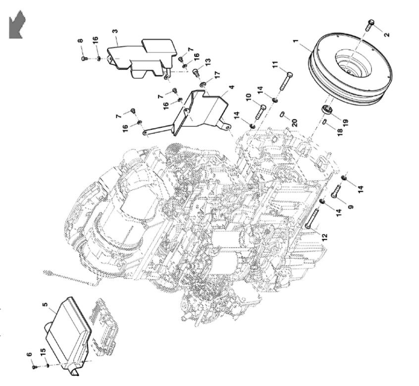
John Deere > Turf And Utility >TRACTOR >F5DFL413T - TRACTOR >5090G Tractor (Engine F5D) IT4 (Europe Edition) >20 ENGINE >ST782264 - MOUNTING PARTS, ENGINE / FLYWHEEL
