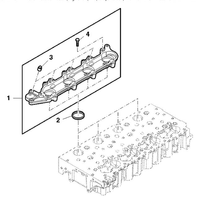
John Deere > Turf And Utility >TRACTOR >F5DFL413T - TRACTOR >5090G Tractor (Engine F5D) IT4 (Europe Edition) >20 ENGINE >ST774083 - CYLINDER HEAD HOUSING
