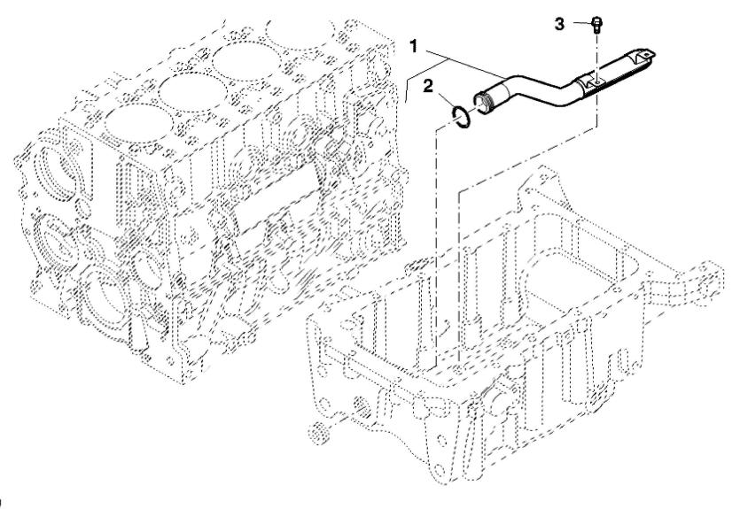
John Deere > Turf And Utility >TRACTOR >F5DFL413T - TRACTOR >5090G Tractor (Engine F5D) IT4 (Europe Edition) >20 ENGINE >ST774119 - SUCTION HOSE
