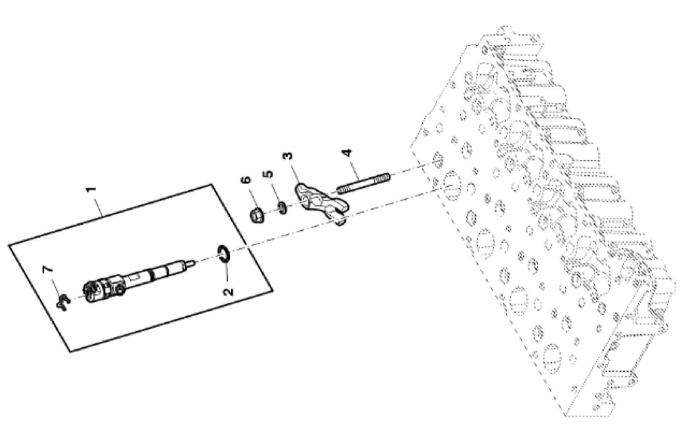
John Deere > Turf And Utility >TRACTOR >F5DFL413T - TRACTOR >5090G Tractor (Engine F5D) IT4 (Europe Edition) >20 ENGINE >ST776357 - INJECTION NOZZLE
