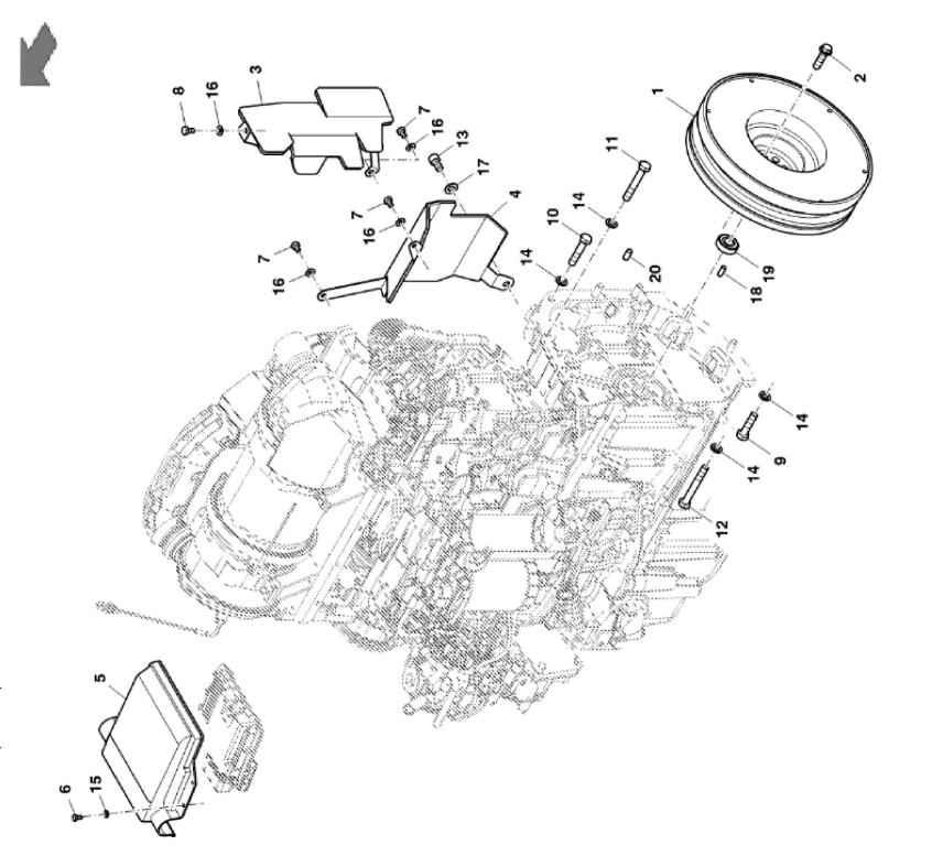
John Deere > Turf And Utility >TRACTOR >F5DFL413S - TRACTOR >5080G Tractor (Engine F5D) IT4 (Europe Edition) >20 ENGINE >ST782264 - MOUNTING PARTS, ENGINE / FLYWHEEL
