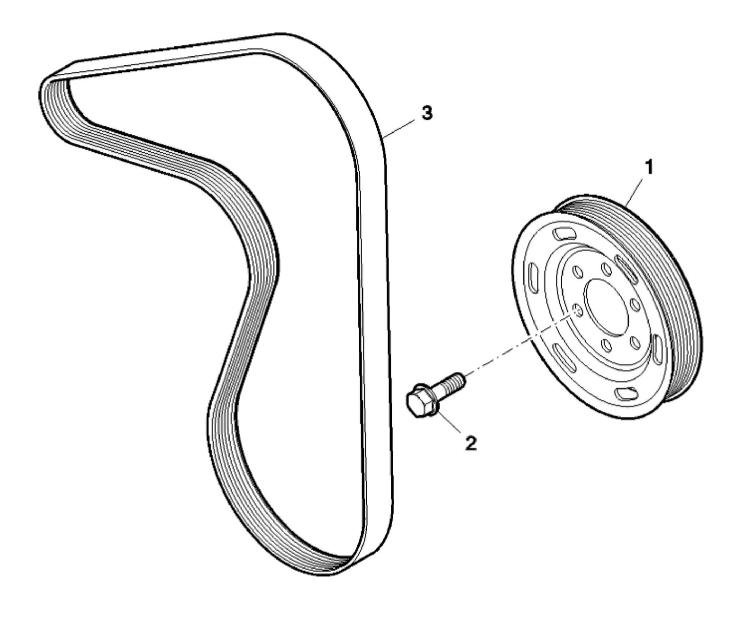
John Deere > Turf And Utility >TRACTOR >F5DFL413S - TRACTOR >5080G Tractor (Engine F5D) IT4 (Europe Edition) >20 ENGINE >ST774090 - DRIVE BELT / PULLEY
