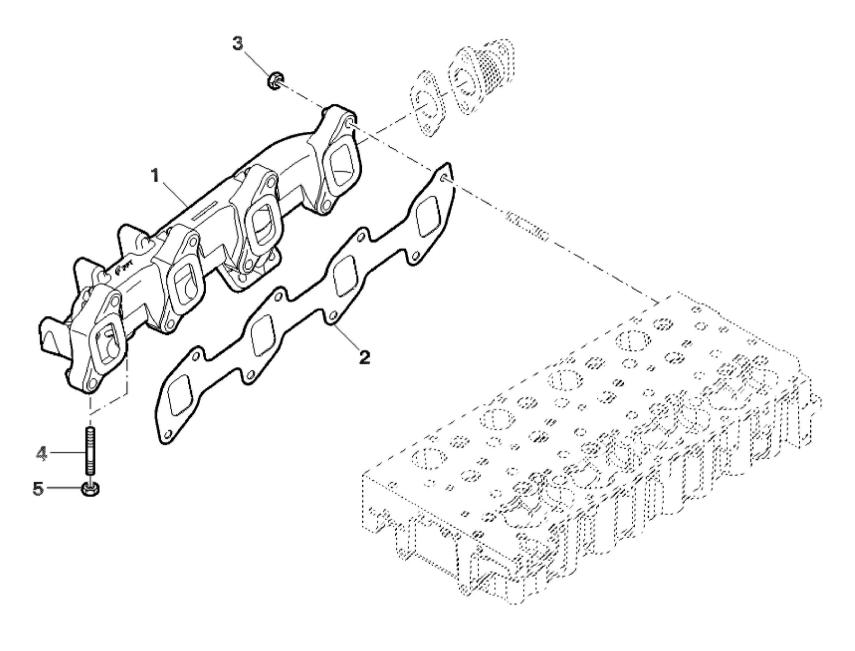
John Deere > Turf And Utility >TRACTOR >F5DFL413S - TRACTOR >5080G Tractor (Engine F5D) IT4 (Europe Edition) >20 ENGINE >ST793021 - EXHAUST MANIFOLD
