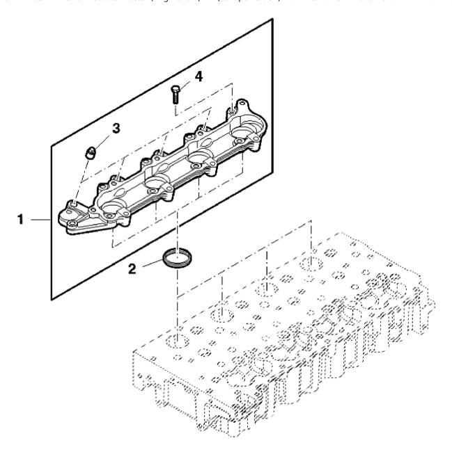
John Deere > Turf And Utility >TRACTOR >F5DFL413S - TRACTOR >5080G Tractor (Engine F5D) IT4 (Europe Edition) >20 ENGINE >ST774083 - CYLINDER HEAD HOUSING
