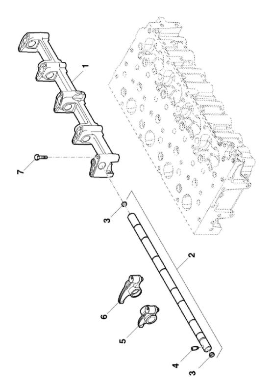
John Deere > Turf And Utility >TRACTOR >F5DFL413S - TRACTOR >5080G Tractor (Engine F5D) IT4 (Europe Edition) >20 ENGINE >ST775005 - ROCKER ARM / SHAFT
