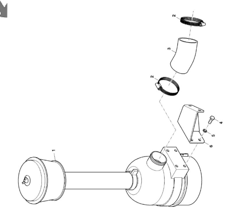
John Deere > Turf And Utility >TRACTOR >B550 - TRACTOR >B550 Tractor >30 FUEL AND AIR >ST257548 - AIR FILTER ASSEMBLY
