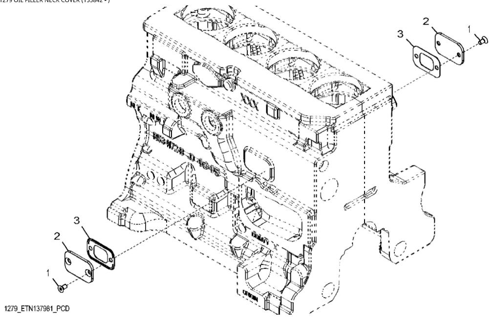
John Deere > Turf And Utility > TRACTOR > 6170M - TRACTOR > 6170M Tractor (Europe Edition, Engine SN: 6068GXXXXXXX)(Tier 2)(S.N. -860503) > 20 ENGINE 6068HL286-DD22382-ETN108063 > ST852078 - 1279 OIL FILLER NECK COVER (155842 - )
