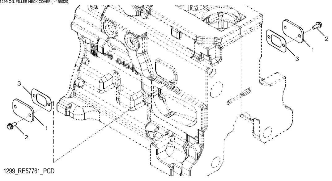
John Deere > Turf And Utility > TRACTOR > 6170M - TRACTOR > 6170M Tractor (Europe Edition, Engine SN: 6068GXXXXXXX)(Tier 2)(S.N. -860503) > 20 ENGINE 6068HL286-DD22382-ETN108063 > ST852076 - 1299 OIL FILLER NECK COVER ( - 155820)
