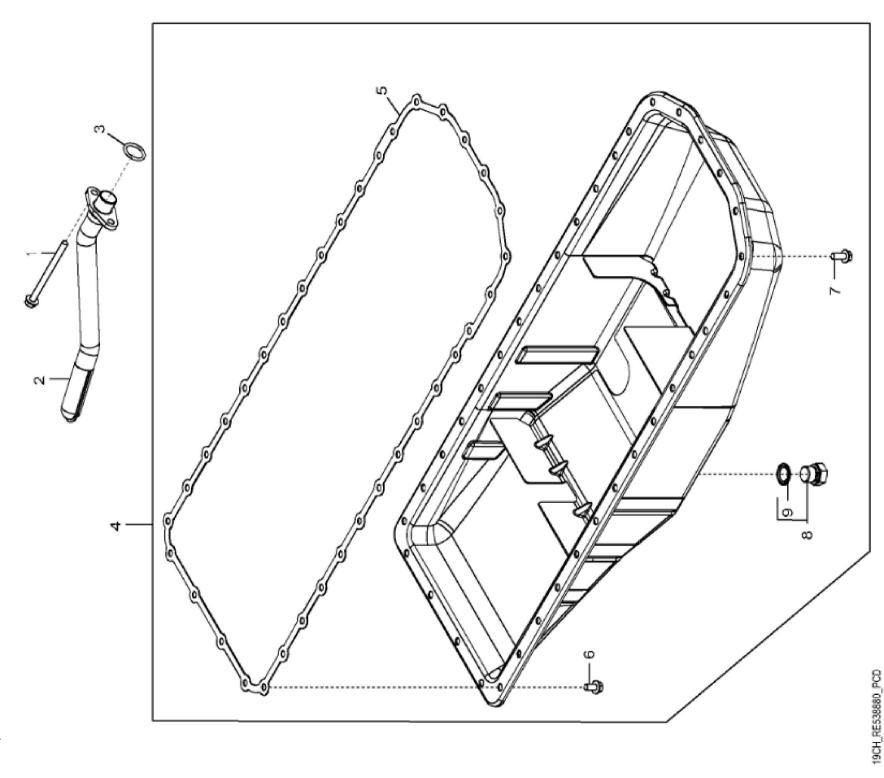
John Deere > Turf And Utility >TRACTOR >6170M - TRACTOR >6170M Tractor (Europe Edition, Engine SN: 6068GXXXXXX)(Tier 2)(S.N. -860503) >20 ENGINE 6068HL286-DD22382-ETN108063 >ST711844 - 19CH OIL PAN
