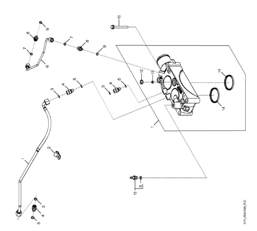
John Deere > Turf And Utility >TRACTOR >6170M - TRACTOR >6170M Tractor (North America Edition, Engine SN: 6068RXXXXXX)(Interim Tier 4) >20 ENGINE 6068HL490-DD22146-ETN65508-ETN68088-ETN65510-ETN74309 >ST261980 - 2174 THERMOSTAT COVER
