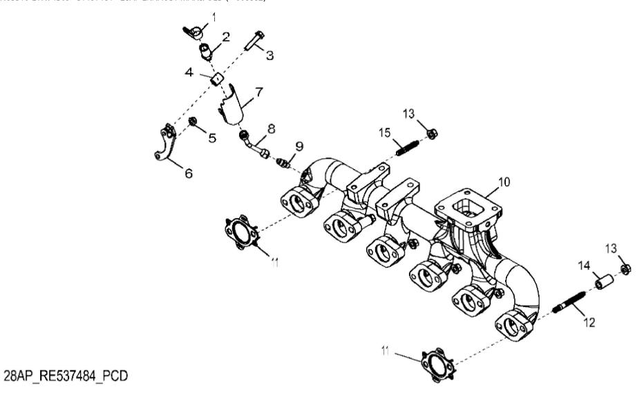
John Deere > Turf And Utility > TRACTOR > 6170M - TRACTOR > 6170M Tractor (North America Edition, Engine SN: 6068RXXXXXXX)(Interim Tier 4) > 20 ENGINE 6068HL490-DD22146-ETN65508-ETN68088-ETN65510-ETN74309 > ST197181 - 28AP EXHAUST MANIFOLD ( - 006882)
