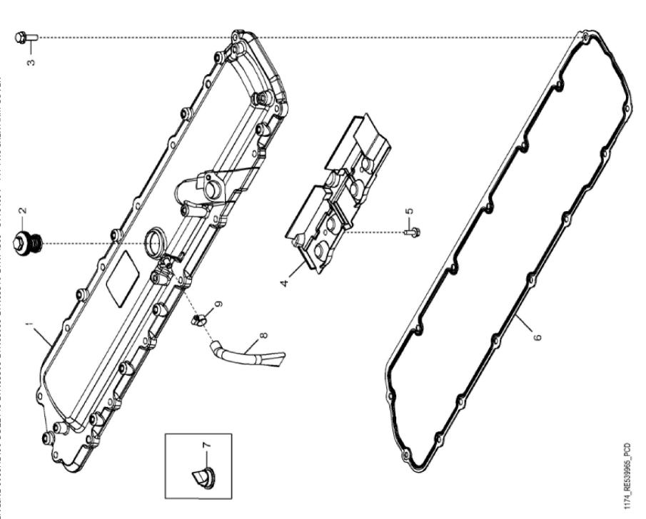
John Deere > Turf And Utility >TRACTOR >6170M - TRACTOR >6170M Tractor (Europe Edition, Engine SN: 6068RXXXXXX)(Interim Tier 4) >20 ENGINE 6068HL490-DD22146-ETN65508-ETN68088-ETN65510-ETN74309 >ST164694 - 1174 ROCKER ARM COVER
