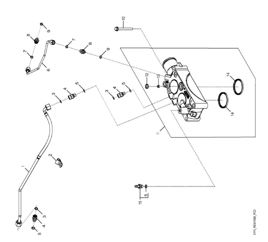
John Deere > Turf And Utility >TRACTOR >6170M - TRACTOR >6170M Tractor (Europe Edition, Engine SN: 6068RXXXXXXX)(Interim Tier 4) >20 ENGINE 6068HL490-DD22146-ETN65508-ETN68088-ETN65510-ETN74309 >ST261980 - 2174 THERMOSTAT COVER
