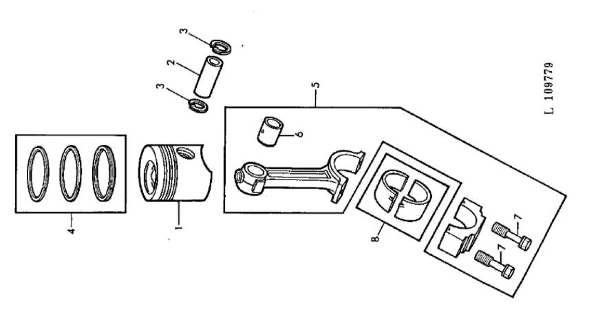
John Deere > Turf And Utility >TRACTOR >820 - TRACTOR >820, 920 Tractors >20 ENGINE >20-18 - PISTON/CONNECTING ROD [01A22]
