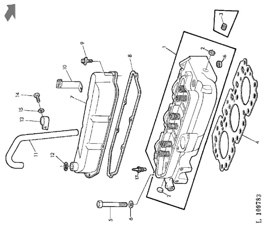
John Deere > Turf And Utility >TRACTOR >820 - TRACTOR >820, 920 Tractors >20 ENGINE >20-8 - CYLINDER HEAD/ROCKER ARM COVER [01A12]
