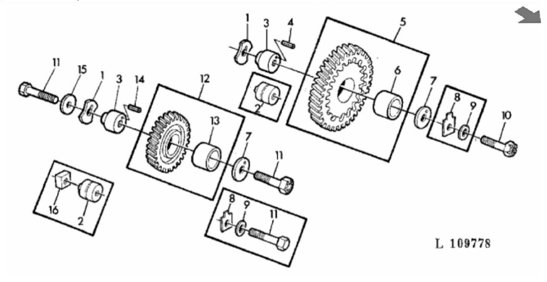
John Deere > Turf And Utility >TRACTOR >820 - TRACTOR >820, 920 Tractors >20 ENGINE >20-17 - TIMING GEARS [01A21]
