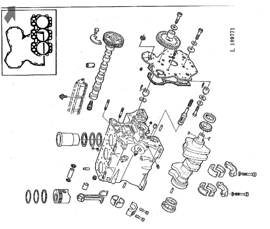
John Deere > Turf And Utility >TRACTOR >820 - TRACTOR >820, 920 Tractors >20 ENGINE >20-2 - SHORT BLOCK ASSEMBLY [01A06]
