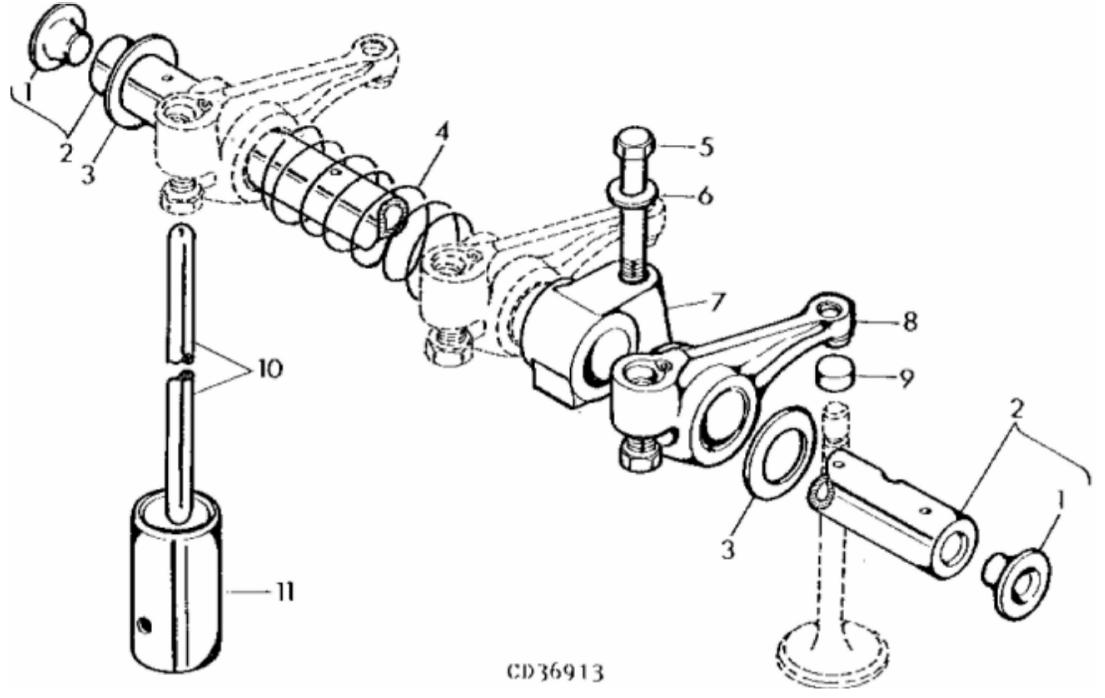
John Deere > Turf And Utility >TRACTOR >830 - TRACTOR >830, 930 Tractors (European Edition) >20 ENGINE >20-13 - ROCKER ARM/SHAFT/TAPPET/PUSH ROD [01A19]
