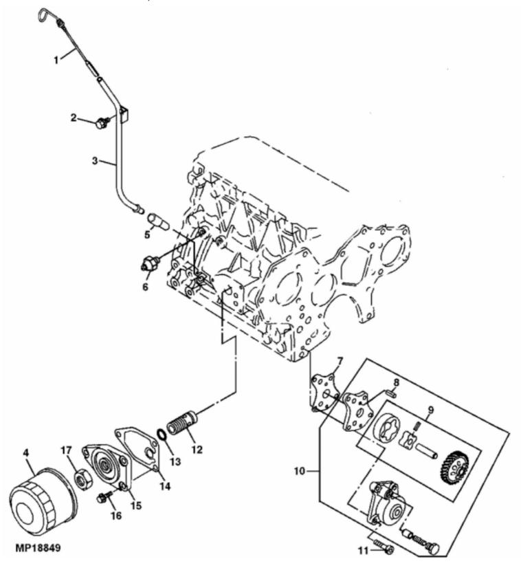
John Deere > Turf And Utility >TRACTOR, COMPACT UTILITY >4610 - TRACTOR, COMPACT UTILITY >4610 Compact Utility Tractor >20 ENGINE >ST641861 - ENGINE OIL PUMP, FILTER AND DIPSTICK
