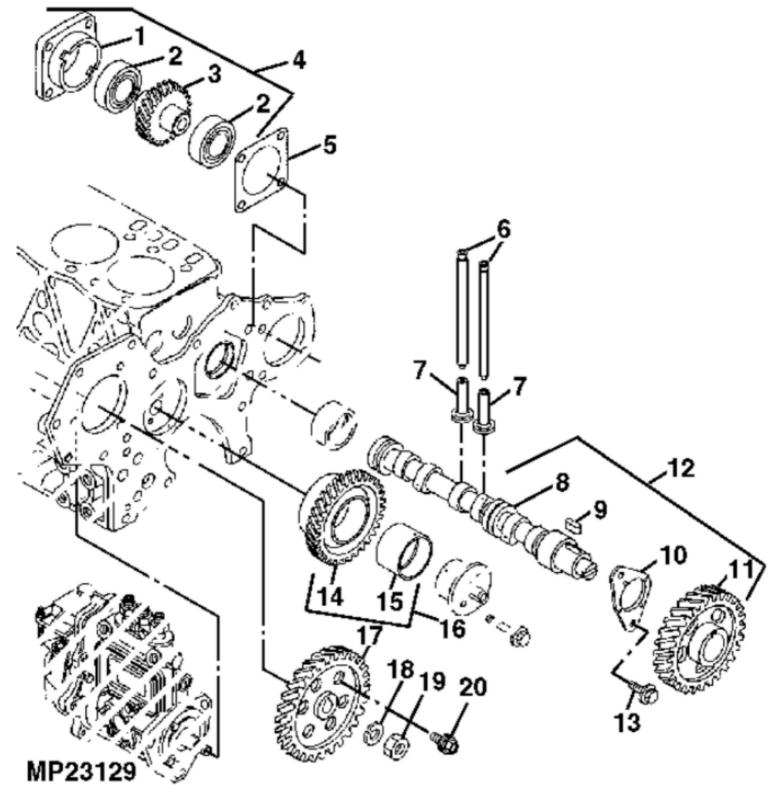
John Deere > Turf And Utility >TRACTOR, COMPACT UTILITY >4410 - TRACTOR, COMPACT UTILITY >4410 Compact Utility Tractor >20 ENGINE >ST641365 - CAMSHAFT AND DRIVING GEARS
