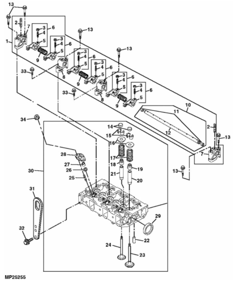
John Deere > Turf And Utility >TRACTOR, COMPACT UTILITY >4410 - TRACTOR, COMPACT UTILITY >4410 Compact Utility Tractor >20 ENGINE >ST641363 - CYLINDER HEAD, VALVES AND ROCKER ARMS
