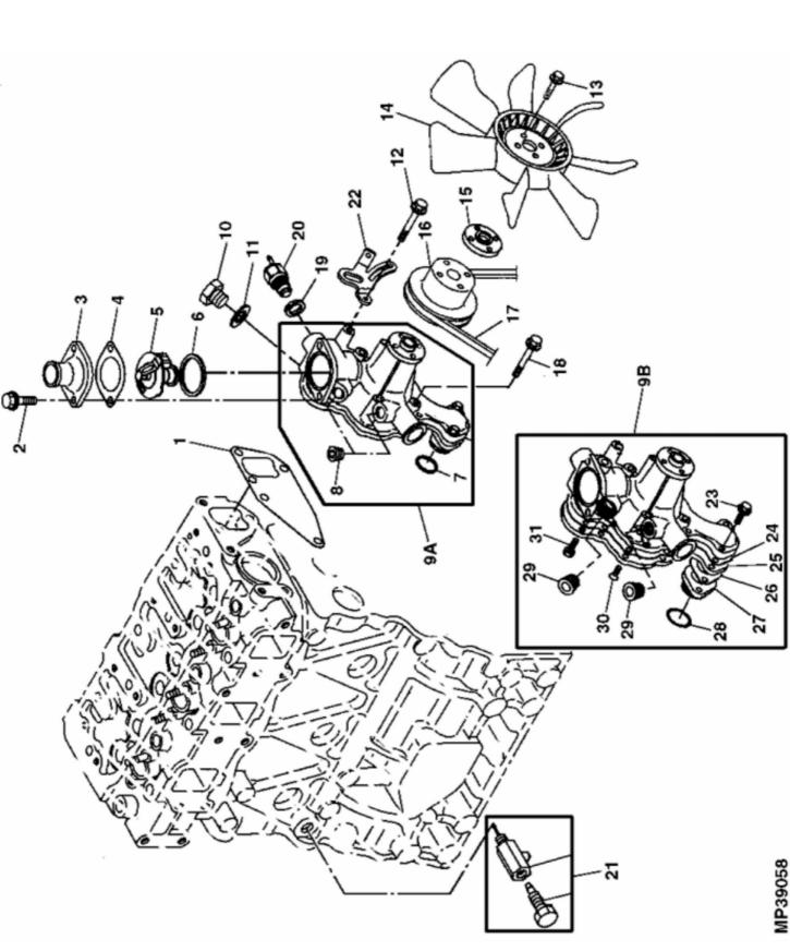
John Deere > Turf And Utility >TRACTOR, COMPACT UTILITY >4410 - TRACTOR, COMPACT UTILITY >4410 Compact Utility Tractor >20 ENGINE >ST641372 - WATER PUMP, THERMOSTAT AND FAN
