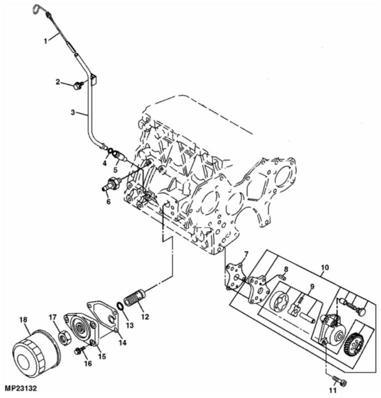
John Deere > Turf And Utility >TRACTOR, COMPACT UTILITY >4410 - TRACTOR, COMPACT UTILITY >4410 Compact Utility Tractor >20 ENGINE >ST641594 - ENGINE OIL PUMP, FILTER / DIPSTICK
