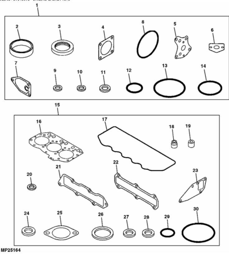
John Deere > Turf And Utility >TRACTOR, COMPACT UTILITY >4210 - TRACTOR, COMPACT UTILITY >4210 Compact Utility Tractor >20 ENGINE >ST640973 - ENGINE GASKET KITS
