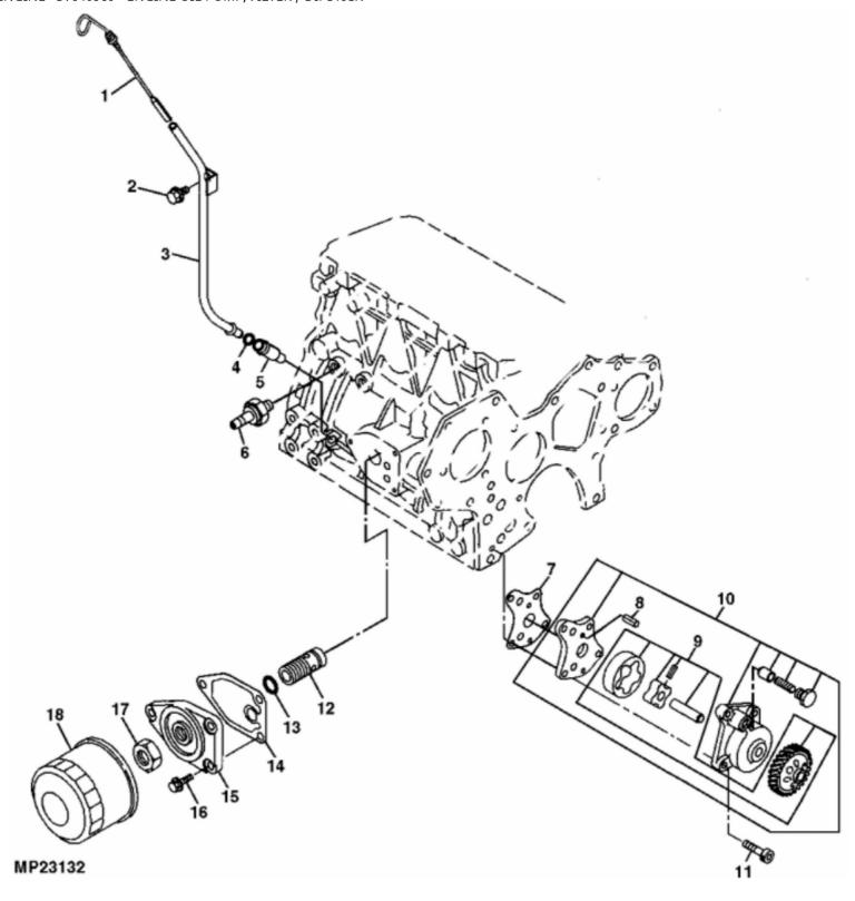
John Deere > Turf And Utility >TRACTOR, COMPACT UTILITY >4210 - TRACTOR, COMPACT UTILITY >4210 Compact Utility Tractor >20 ENGINE >ST640969 - ENGINE OIL PUMP, FILTER / DIPSTICK
