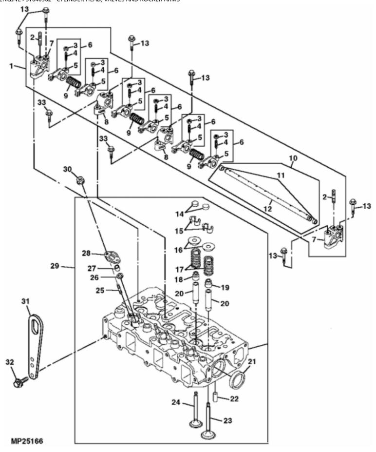
John Deere > Turf And Utility >TRACTOR, COMPACT UTILITY >4210 - TRACTOR, COMPACT UTILITY >4210 Compact Utility Tractor >20 ENGINE >ST640962 - CYLINDER HEAD, VALVES AND ROCKER ARMS
