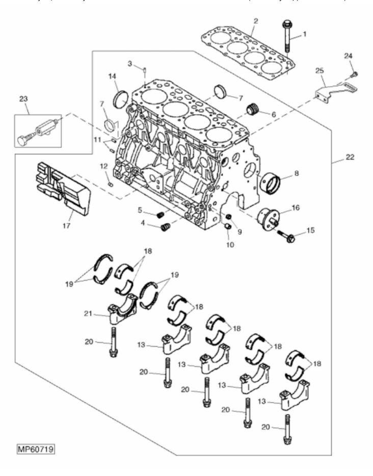
John Deere > Turf And Utility > BACKHOE, LOADER > 110 - BACKHOE, LOADER > 110 Tractor Loader Backhoe (Worldwide Edition) > 20 ENGINE 4TNE84-EJTLB, 4TNV88-MJTLB > ST151418 - CYLINDER
