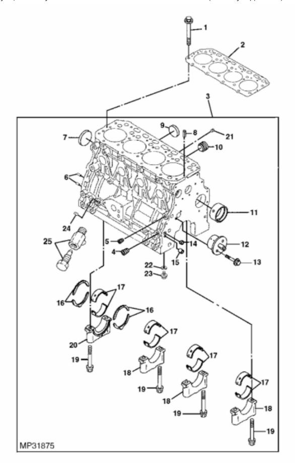
John Deere > Turf And Utility > BACKHOE, LOADER > 110 - BACKHOE, LOADER > 110 Tractor Loader Backhoe (Worldwide Edition) > 20 ENGINE 4TNE84-EJTLB, 4TNV88-MJTLB > ST151417 - CYLINDER BLOCK AND MAIN BEARINGS (4TNE84-EJTLB) ( - 311032)
