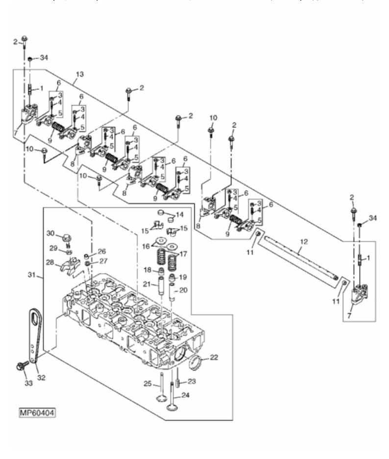
John Deere > Turf And Utility > BACKHOE, LOADER > 110 - BACKHOE, LOADER > 110 Tractor Loader Backhoe (Worldwide Edition) > 20 ENGINE 4TNE84-EJTLB, 4TNV88-MJTLB > ST151420 - CYLINDER
