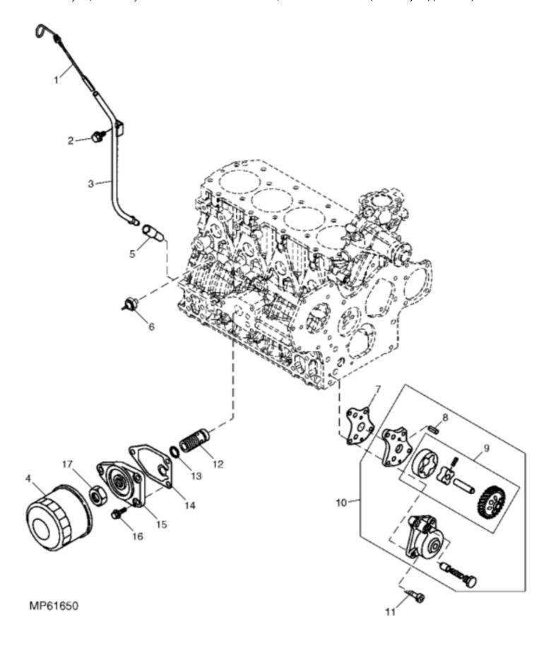
John Deere > Turf And Utility > BACKHOE, LOADER > 110 - BACKHOE, LOADER > 110 Tractor Loader Backhoe (Worldwide Edition) > 20 ENGINE 4TNE84-EJTLB, 4TNV88-MJTLB > ST151431 - ENGINE OIL PUMP, FILTER AND DIPSTICK (4TNE84-EJTLB) ( - 311032)
