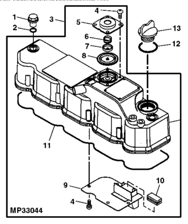
John Deere > Turf And Utility >TRACTOR, COMPACT UTILITY >990 - TRACTOR, COMPACT UTILITY >990 Compact Utility Tractor >20 ENGINE >ST540596 - CYLINDER HEAD COVER AND GASKETS
