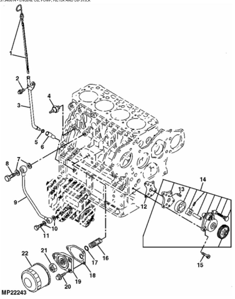
John Deere > Turf And Utility >TRACTOR, COMPACT UTILITY >990 - TRACTOR, COMPACT UTILITY >990 Compact Utility Tractor >20 ENGINE >ST540614 - ENGINE OIL PUMP, FILTER AND DIPSTICK
