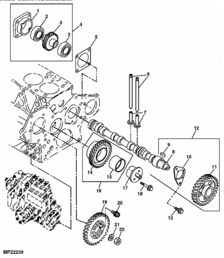
John Deere > Turf And Utility > TRACTOR, COMPACT UTILITY > 990 - TRACTOR, COMPACT UTILITY > 990 Compact Utility Tractor > 20 ENGINE > ST540598 - CAMSHAFT AND DRIVING GEARS
