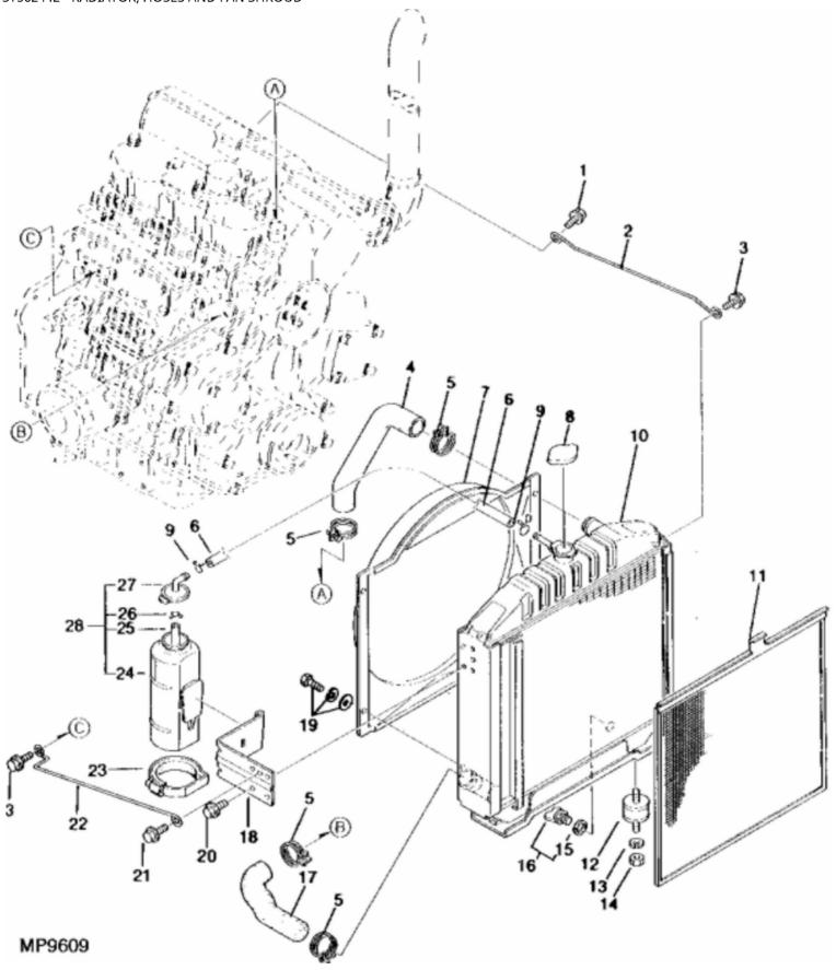
John Deere > Turf And Utility >TRACTOR, COMPACT UTILITY >790 - TRACTOR, COMPACT UTILITY >790 Compact Utility Tractor >20 ENGINE >ST562442 - RADIATOR, HOSES AND FAN SHROUD
