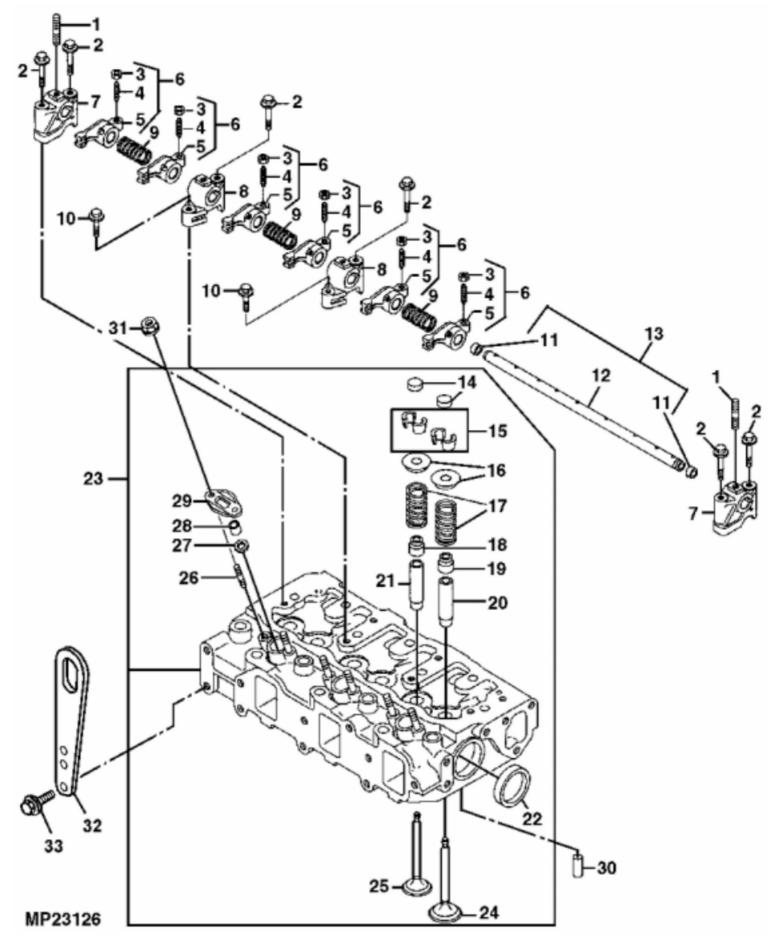
John Deere > Turf And Utility > TRACTOR, COMPACT UTILITY > 790 - TRACTOR, COMPACT UTILITY > 790 Compact Utility Tractor > 20 ENGINE > ST562432 - CYLINDER HEAD, VALVES AND ROCKER ARMS
