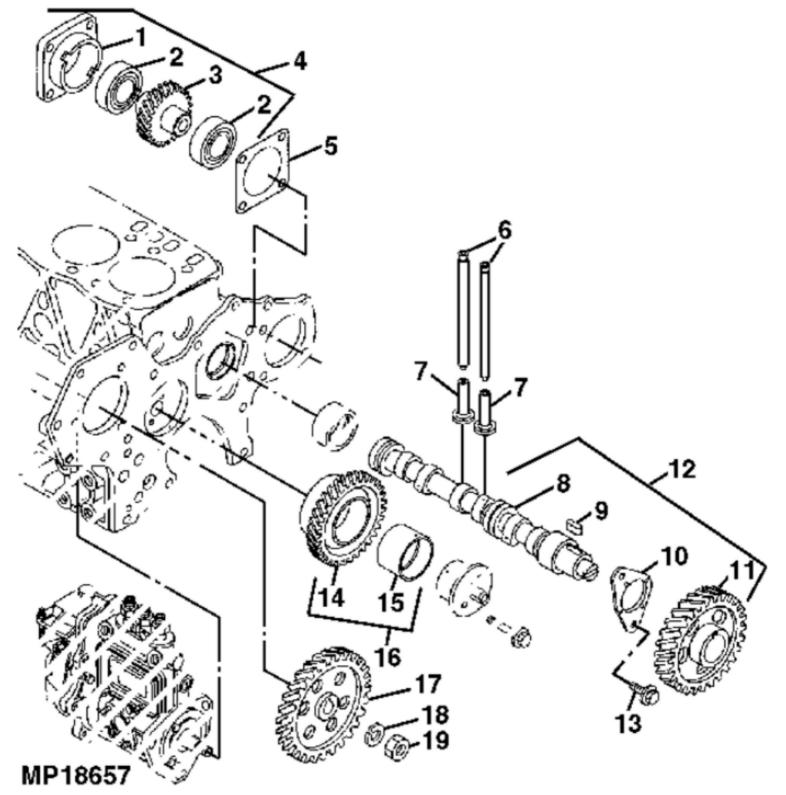
John Deere > Turf And Utility >TRACTOR, COMPACT UTILITY >790 - TRACTOR, COMPACT UTILITY >790 Compact Utility Tractor >20 ENGINE >ST562434 - CAMSHAFT AND DRIVING GEARS
