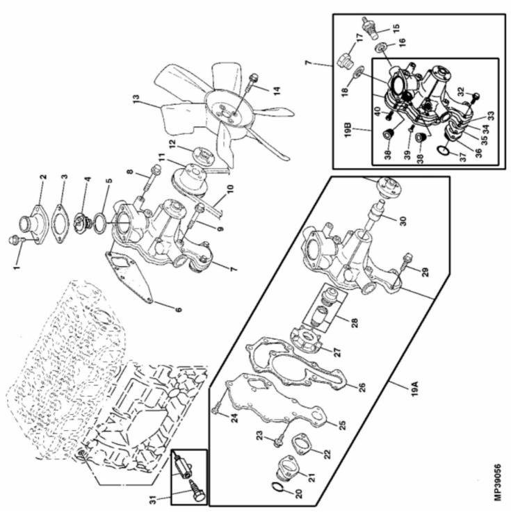
John Deere > Turf And Utility >TRACTOR, COMPACT UTILITY >790 - TRACTOR, COMPACT UTILITY >790 Compact Utility Tractor >20 ENGINE >ST562441 - WATER PUMP, THERMOSTAT AND FAN
