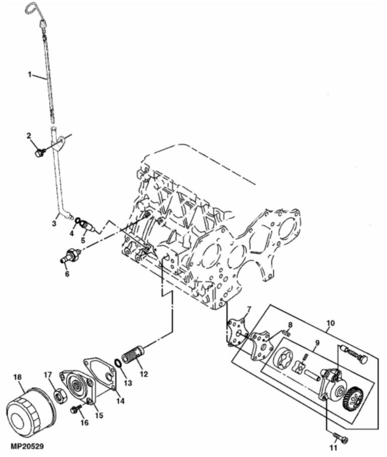
John Deere > Turf And Utility >TRACTOR, COMPACT UTILITY >790 - TRACTOR, COMPACT UTILITY >790 Compact Utility Tractor >20 ENGINE >ST562439 - ENGINE OIL PUMP, FILTER / DIPSTICK
