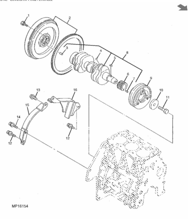
John Deere > Turf And Utility >TRACTOR, COMPACT UTILITY >955 - TRACTOR, COMPACT UTILITY >955 Compact Utility Tractor >20 ENGINE >ST553149 - CRANKSHAFT AND FLYWHEEL
