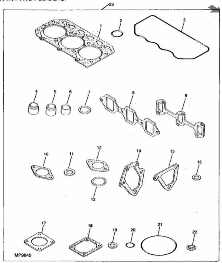
John Deere > Turf And Utility >TRACTOR, COMPACT UTILITY >955 - TRACTOR, COMPACT UTILITY >955 Compact Utility Tractor >20 ENGINE >ST553153 - CYLINDER HEAD GASKET KIT
