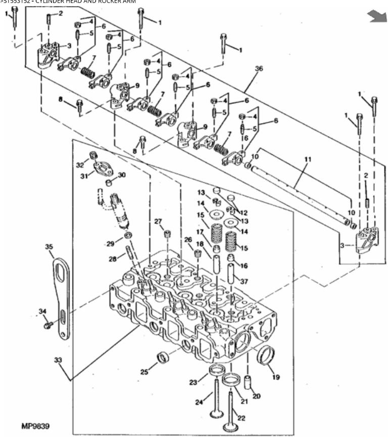
John Deere > Turf And Utility >TRACTOR, COMPACT UTILITY >955 - TRACTOR, COMPACT UTILITY >955 Compact Utility Tractor >20 ENGINE >ST553152 - CYLINDER HEAD AND ROCKER ARM
