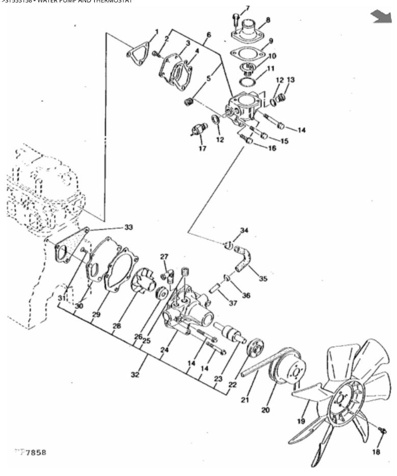
John Deere > Turf And Utility >TRACTOR, COMPACT UTILITY >955 - TRACTOR, COMPACT UTILITY >955 Compact Utility Tractor >20 ENGINE >ST553158 - WATER PUMP AND THERMOSTAT
