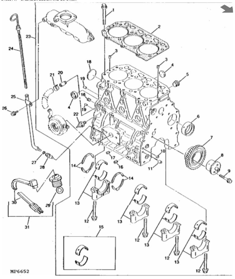
John Deere > Turf And Utility >TRACTOR, COMPACT UTILITY >955 - TRACTOR, COMPACT UTILITY >955 Compact Utility Tractor >20 ENGINE >ST553147 - CYLINDER BLOCK AND DIPSTICK
