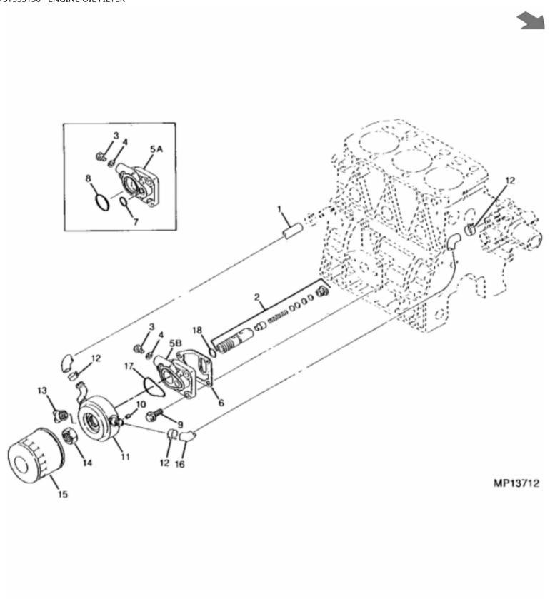
John Deere > Turf And Utility >TRACTOR, COMPACT UTILITY >955 - TRACTOR, COMPACT UTILITY >955 Compact Utility Tractor >20 ENGINE >ST553156 - ENGINE OIL FILTER
