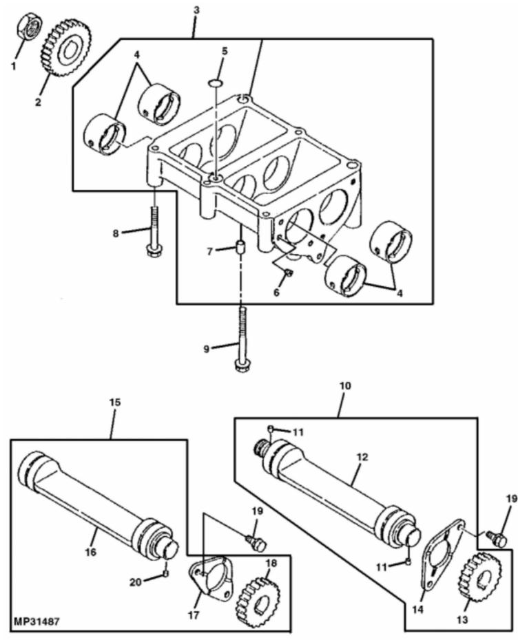
John Deere > Turf And Utility >TRACTOR, COMPACT UTILITY >970 - TRACTOR, COMPACT UTILITY >870, 970 and 1070 Compact Utility Tractors >20 ENGINE >ST632016 - BALANCER (970/1070)
