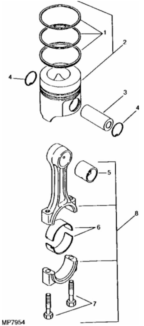
John Deere > Turf And Utility >TRACTOR, COMPACT UTILITY >970 - TRACTOR, COMPACT UTILITY >870, 970 and 1070 Compact Utility Tractors >20 ENGINE >ST632015 - PISTON AND CONNECTING ROD
