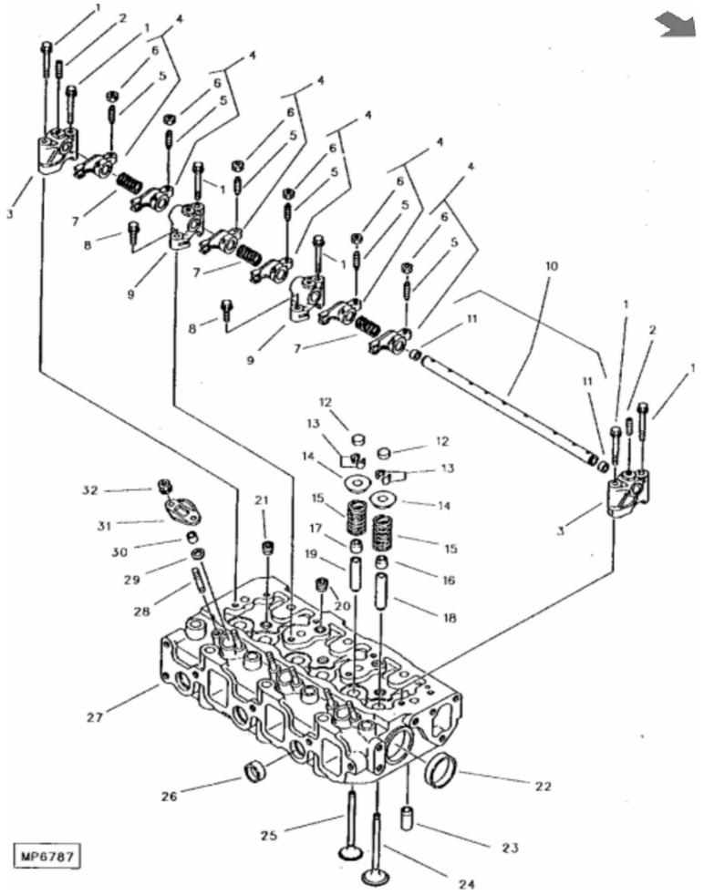
John Deere > Turf And Utility >TRACTOR, COMPACT UTILITY >970 - TRACTOR, COMPACT UTILITY >870, 970 and 1070 Compact Utility Tractors >20 ENGINE >ST632008 - CYLINDER HEAD (870)
