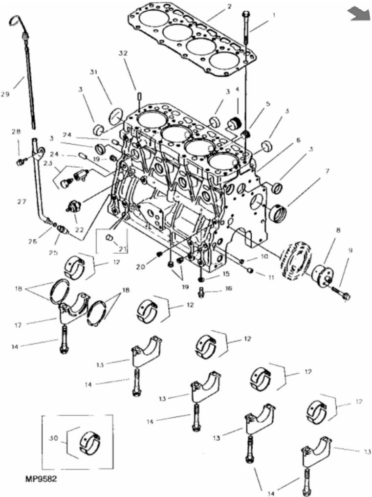
John Deere > Turf And Utility >TRACTOR, COMPACT UTILITY >970 - TRACTOR, COMPACT UTILITY >870, 970 and 1070 Compact Utility Tractors >20 ENGINE >ST632012 - CYLINDER BLOCK (970/1070)
