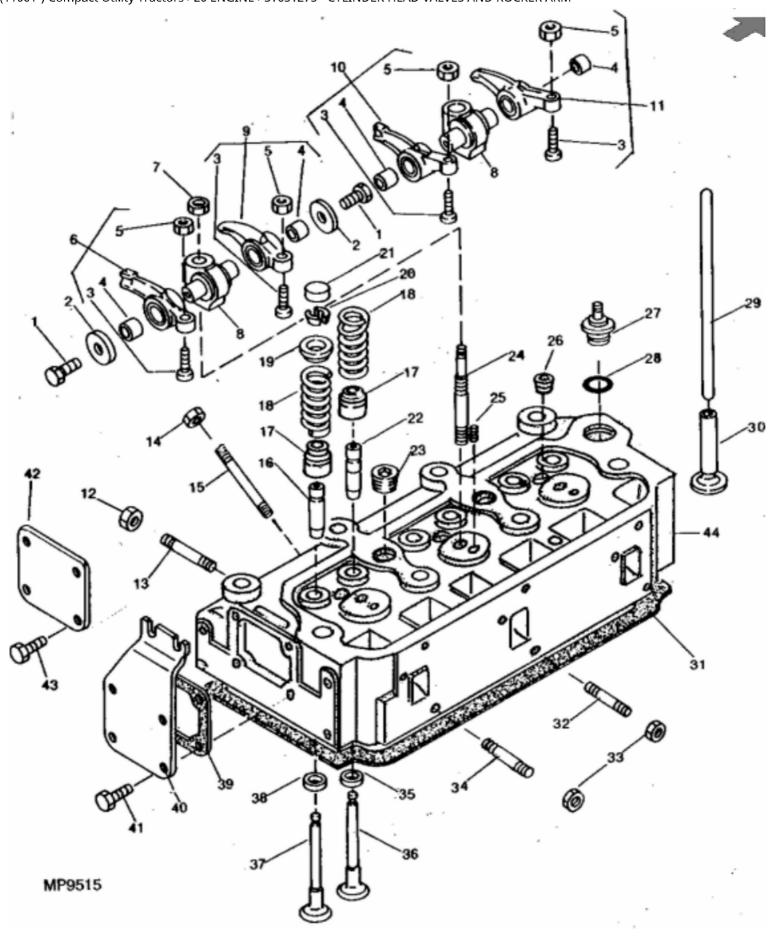
John Deere > Turf And Utility >TRACTOR, COMPACT UTILITY >950 - TRACTOR, COMPACT UTILITY >850 (16001-), 950 (20001-) and 1050 (11001-) Compact Utility Tractors >20 ENGINE >ST631275 -
