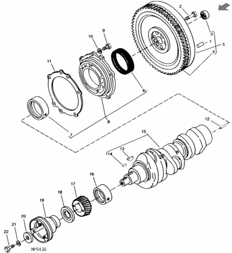
John Deere > Turf And Utility > TRACTOR, COMPACT UTILITY >950 - TRACTOR, COMPACT UTILITY >850 ( -16000) & 950 ( -20000) Compact Utility Tractors >20 ENGINE >ST631039 - CRANKSHAFT AND FLYWHEEL (3T80J) (850)
