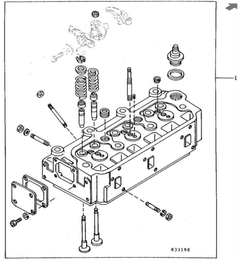
John Deere > Turf And Utility > TRACTOR, COMPACT UTILITY >950 - TRACTOR, COMPACT UTILITY >850 ( -16000) & 950 ( -20000) Compact Utility Tractors >20 ENGINE >ST631030 - CYLINDER HEAD (3T80J) (850)
