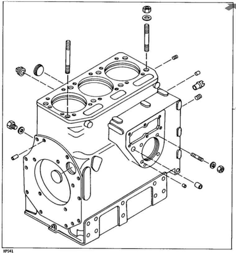
John Deere > Turf And Utility > TRACTOR, COMPACT UTILITY >950 - TRACTOR, COMPACT UTILITY >850 ( -16000) & 950 ( -20000) Compact Utility Tractors >20 ENGINE >ST631036 - CYLINDER BLOCK (3T80J) (850)
