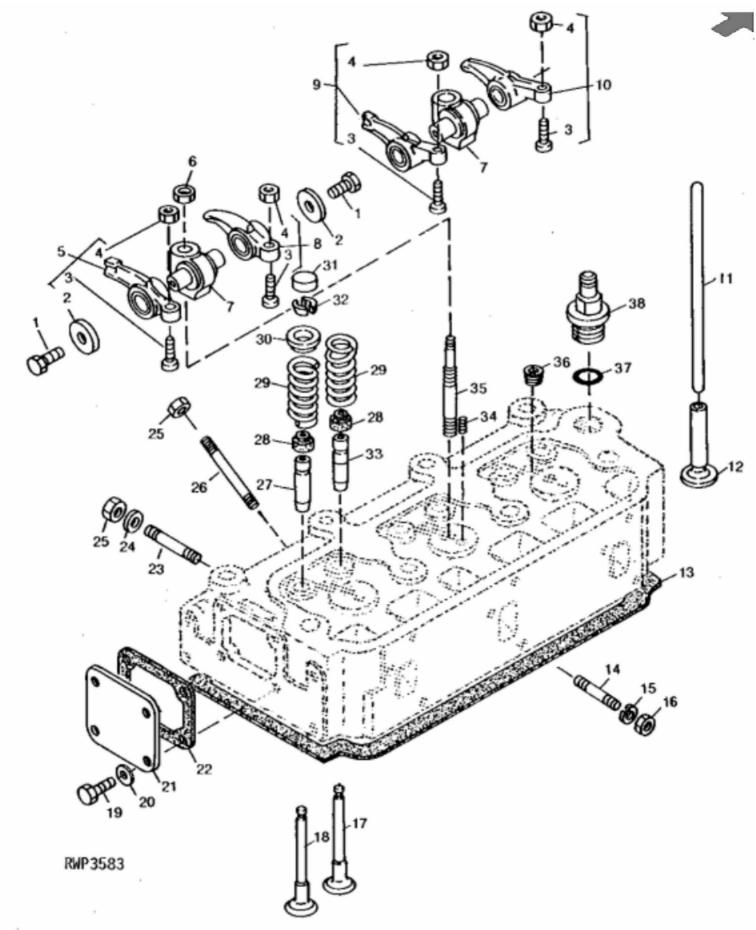
John Deere > Turf And Utility >TRACTOR, COMPACT UTILITY >950 - TRACTOR, COMPACT UTILITY >850 ( -16000) & 950 ( -20000) Compact Utility Tractors >20 ENGINE >ST631029 - CYLINDER HEAD
