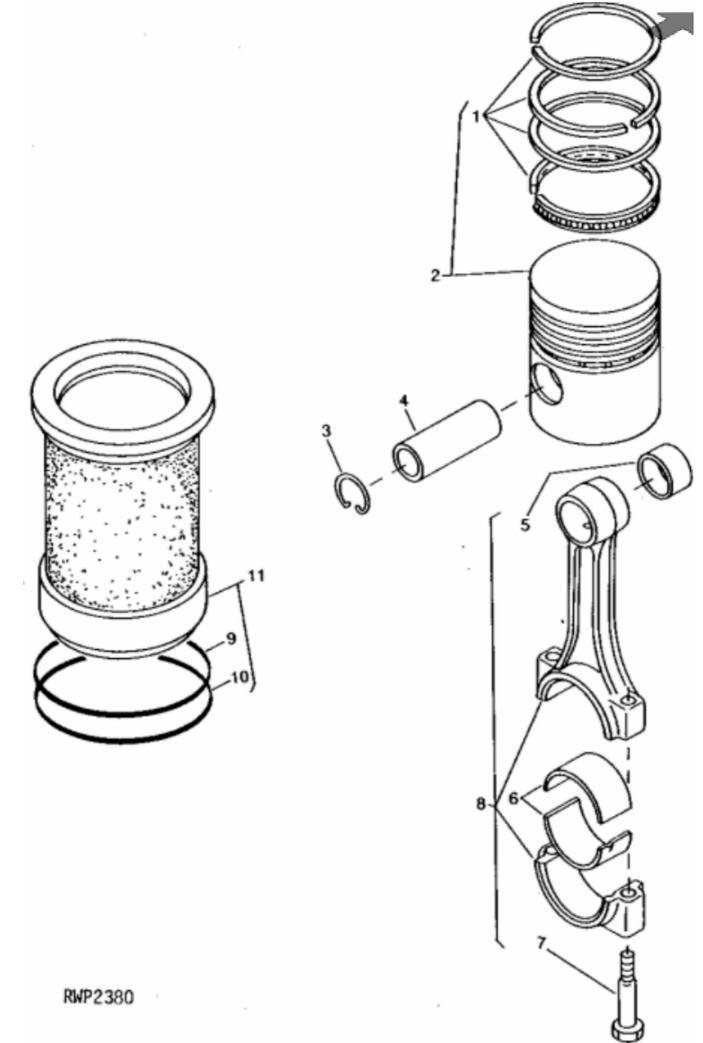
John Deere > Turf And Utility >TRACTOR, COMPACT UTILITY >950 - TRACTOR, COMPACT UTILITY >850 ( -16000) & 950 ( -20000) Compact Utility Tractors >20 ENGINE >ST631038 - PISTON, RINGS AND LINER (3T80J) (850)
