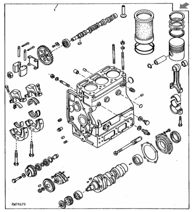
John Deere > Turf And Utility >TRACTOR, COMPACT UTILITY >950 - TRACTOR, COMPACT UTILITY >850 ( -16000) & 950 ( -20000) Compact Utility Tractors >20 ENGINE >ST631037 - SHORT BLOCK ASSEMBLY
